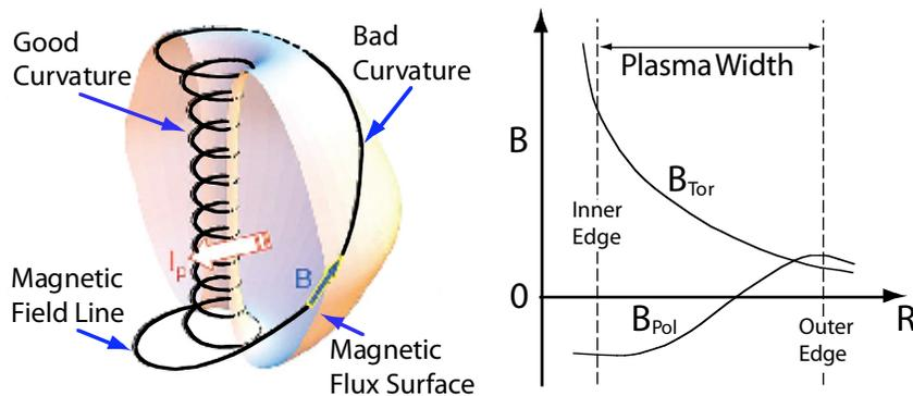
Fig. 5-1. The Spherical Tokamak magnetic configuration. The poloidal field,  $B_p$ , is comparable to the toroidal field,  $B_T$ , near the outboard plasma edge, and much smaller near the inboard plasma edge.
