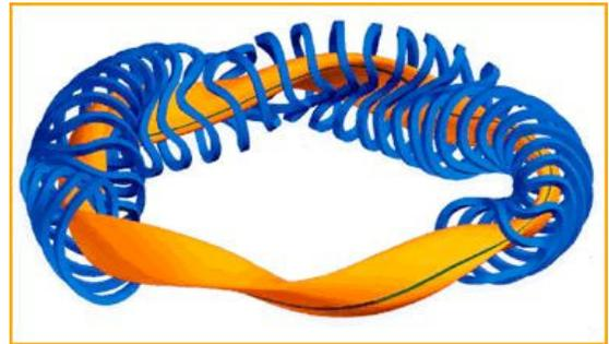
Fig. 4-3. W7-AS modular non-planar coils and plasma.
