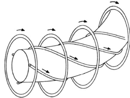
Fig. 4-1. Basic coil configuration for a simple stellarator showing toroidal field coils and helical windings to provide rotational transform.
