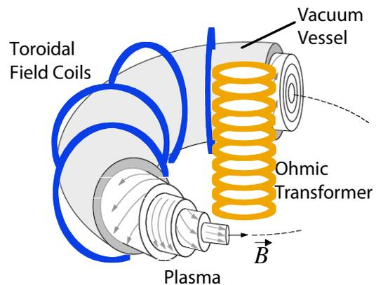
Fig. 2-4. The reversed-field pinch configuration.
