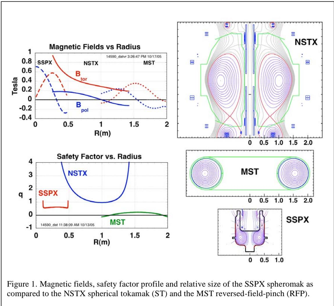
Figure 1. Magnetic fields, safety factor profile and relative size of the SSPX spheromak as compared to the NSTX spherical tokamak (ST) and the MST reversed-field-pinch (RFP).
