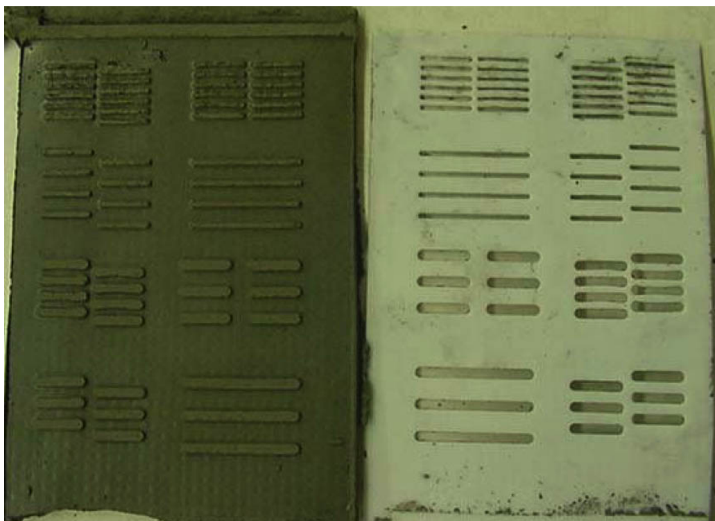
Fig. 4-12. Prototype of a C-SiC microchannel plate. (Photo courtesy of P. Petersen, UC Berkeley.)
