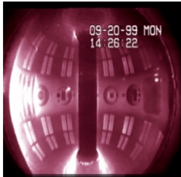
Fig. 2. The spherical torus such as this one at Princeton University, has a central conductor with an extremely small radius and an optimum shape for containing high pressure.
