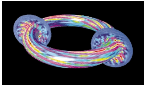
Fig. 4. The computational simulation of plasma turbulence in a tokamak ring was constructed to aid understanding of how turbulence affects heat transfer and hence the efficiency of fusion. (Courtesy of W. Lee and S. Parker, Princeton Plasma Physics Laboratory.)
