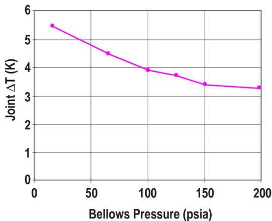
Fig. 5. Thermal performance of liquid nitrogen cooled parting joint as at 1 W conducted heat load.
