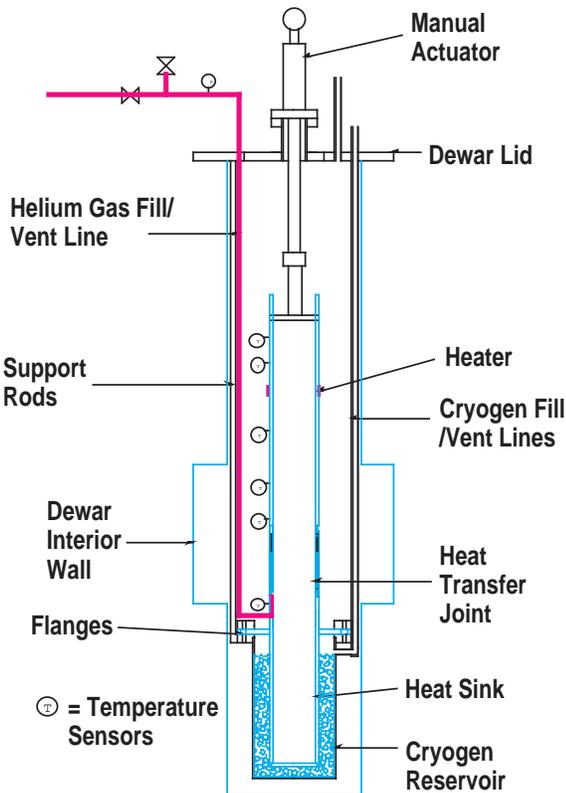
Fig. 3. Test fixture hardware (cross section view).
