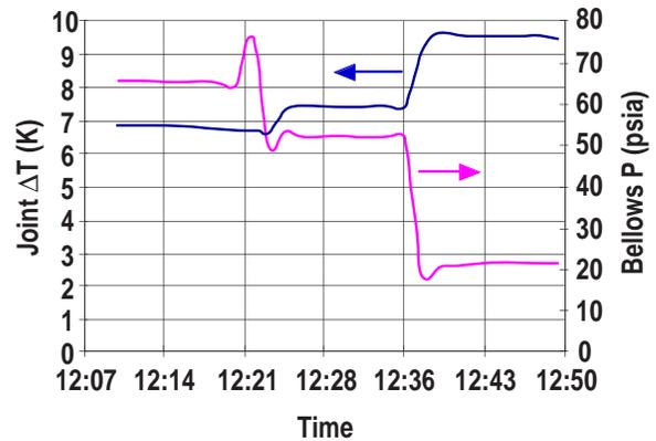
Fig. 9. Typical experimental trace obtained for step changes in bellows pressure while operating at liquid helium temperatures.
