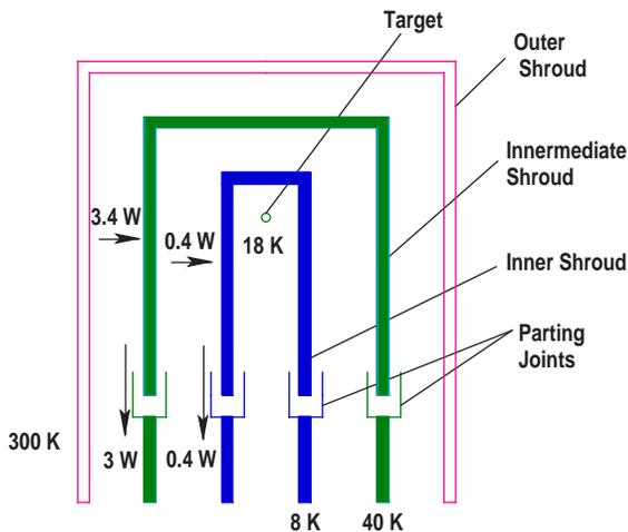
Fig. 2. Moving cryostat shroud assembly diagram.
