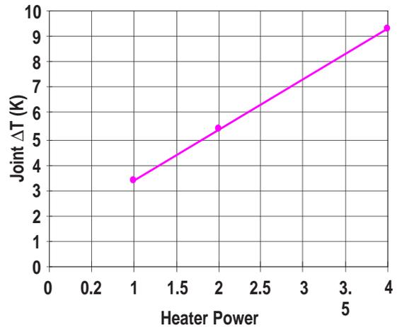
Fig. 6. Thermal performance of liquid helium cooled parting joint at 150 psia bellows pressure.
