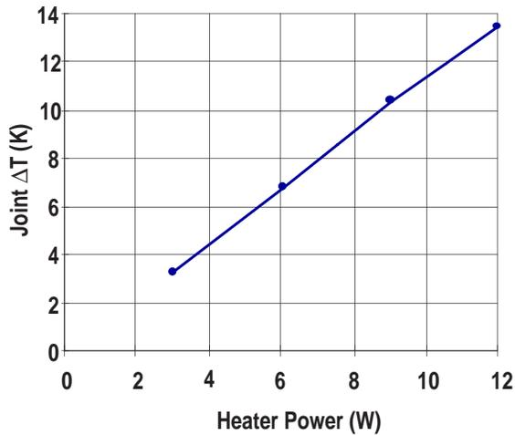
Fig. 8. Thermal performance of liquid nitrogen cooled parting joint at 150 psia bellows pressure.
