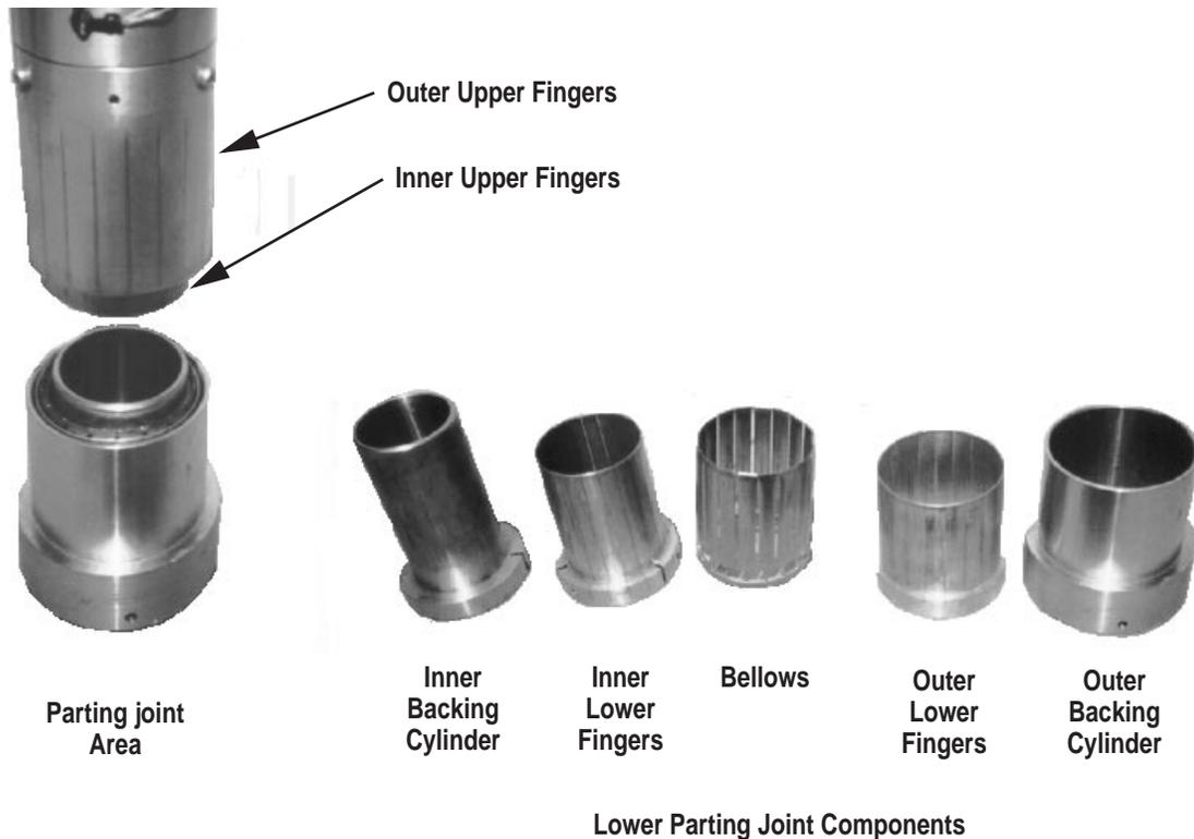
Fig. 1. Cryogenic parting joint prototype.
