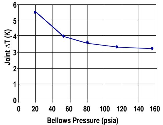
Fig. 7. Thermal performance of liquid nitrogen cooled parting joint at 3 W conducted heat load.
