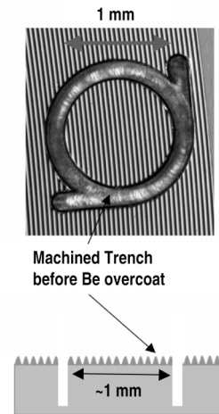
Figure 3. Milled trench to allow access to substrate after over coat.
