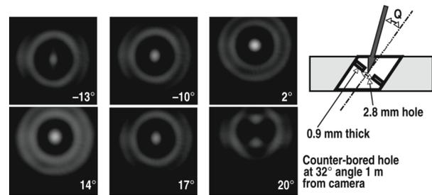
Figure 4. The Fresnel diffraction spots shown are zone 3. The laser wavelength is 632 nm. Zone 3 provides a bright central spot surrounded by a high contrast dark band. Note that the spot is maintained for significantly large tilt angles of the incident laser light.
