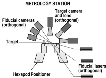
Figure 2. The metrology station is used to establish to offset of the target from the fiducial marks on the carrier. Three orthogonal positioned apertures are used as fiducials. Each target is positioned to the same location in front of the target cameras. The offset of the diffraction spots produced by the lasers on the fiducial cameras is recorded for used by the alignment system on the laser chamber. A hexapod is used to move the target carrier is all six degrees of freedom.
