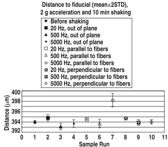
Figure 8. Target to carrier reference fiducial separation did not change after shaking.
