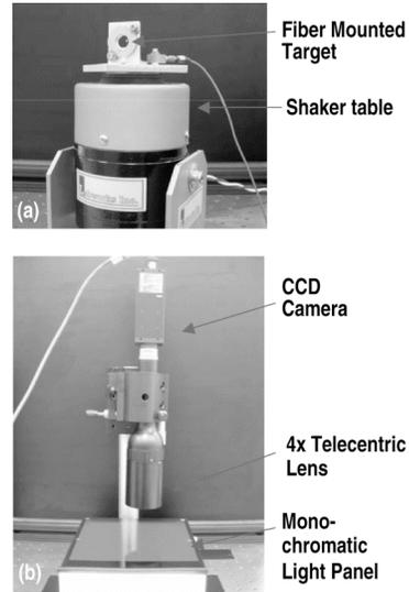
Figure 7. (a) Targets were shaken with a shaker table. (b) Targets were imaged to measure their separation.
