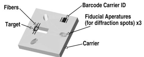
Figure 1. A target carrier is used for each target. Fiducial marks (apertures) are used to align target/carrier assembly to the laser and diagnostics.
