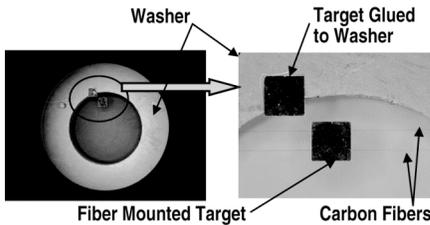
Figure 6. Aluminum targets were mounted using two parallel carbon fibers to a washer. The top target is attached to washer as a reference. The bottom target is glued to the fibers. The corner-to-corner distance between targets is measured. The washer represents the target carrier.
