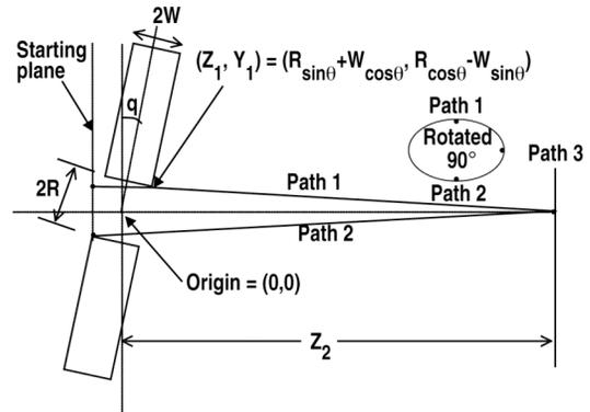
Figure 5. For a tilted aperture (hole), light ray paths have different lengths. Consider light grazing top (path 1), bottom (path 3), and side (path 3), of hole.
