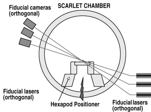
Figure 3. The target carrier is aligned using the diffraction spots produced by the lasers passing through the apertures on the target carrier. The spots are images by the CCD cameras. The offset of the target to the apertures measured previously by the metrology station is applied to bring the target into alignment. The electronic alignment equipment, CCD cameras and lasers, are located outside of the vacuum chamber for reduced EMP exposure.
