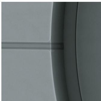
Figure 7. (a) A high magnification x-ray image of a glass fill tube attachment. Fill tube insertion depth, wall thickness, and a small hole cavity are observed in the x-ray image.
