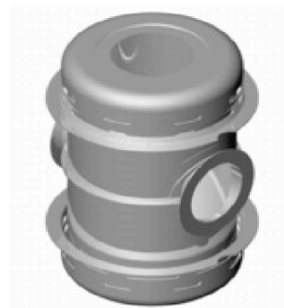
Figure 2. NIF cryogenic hohlraum with window saddles.
