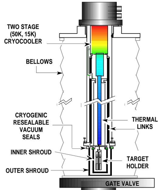
Fig. 3. Prototype cold transfer cryostat.
