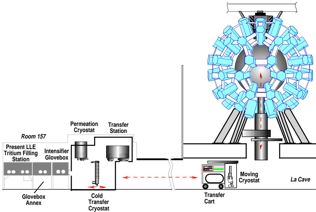
Fig. 1. OMEGA cryogenic target system.
