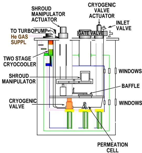
Fig. 2. Prototype permeation cryostat.
