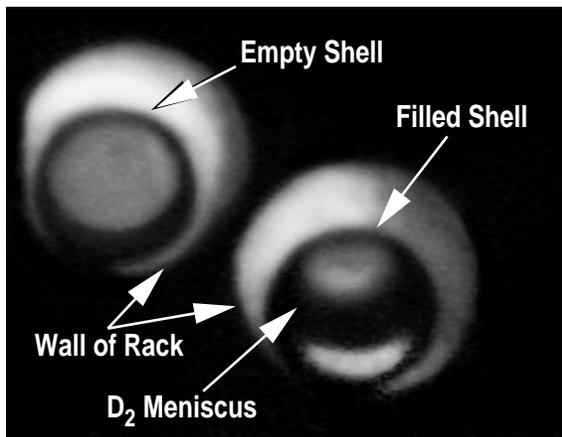
Fig. 4. Filled shells have distinctive appearance (filled shell on right).
