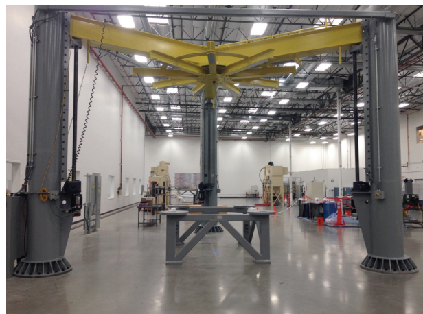
Fig. 2. The tool for supporting and lowering the hex/quad pancakes installed in GA's facility.
