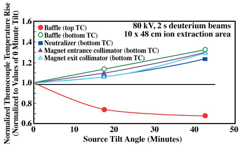
Fig. 5. Normalized temperature rises of collimators vs. source tilt angles.
