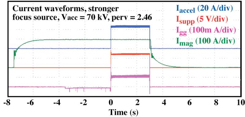
Fig. 8. Waveforms of beam currents.
