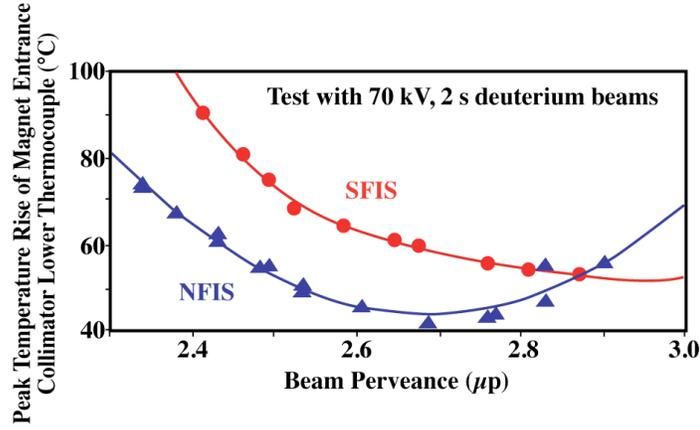
Fig. 10. Magnet entrance collimator temperature rise.
