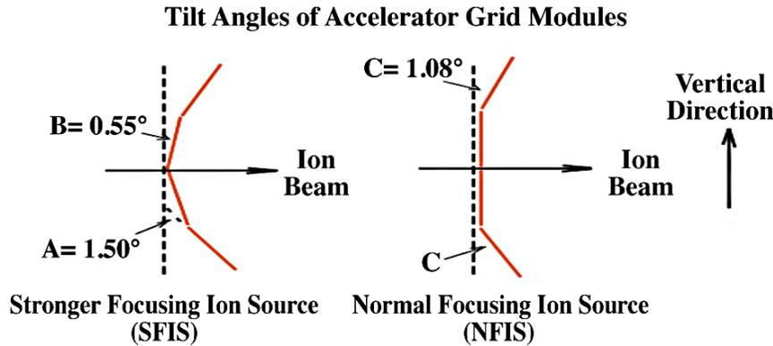
Fig. 6. Tilt angles of accelerator grid modules for SFIS and NFIS.
