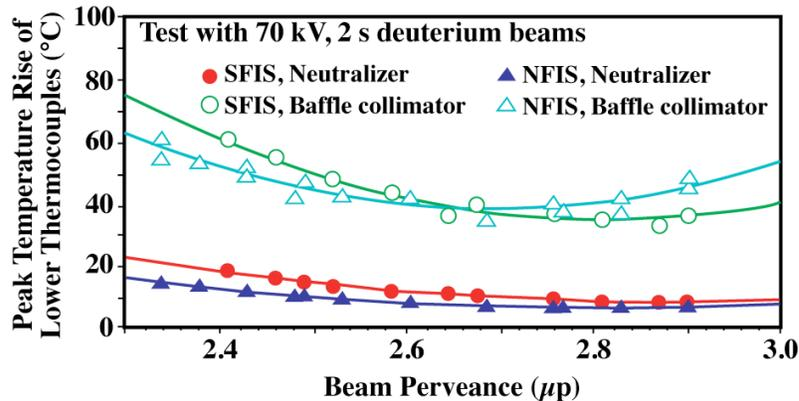
Fig. 9. Neutralizer and baffle collimator temperature rises.
