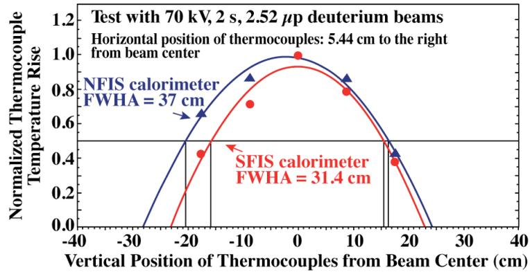
Fig. 16. Vertical beam profiles at the calorimeter.
