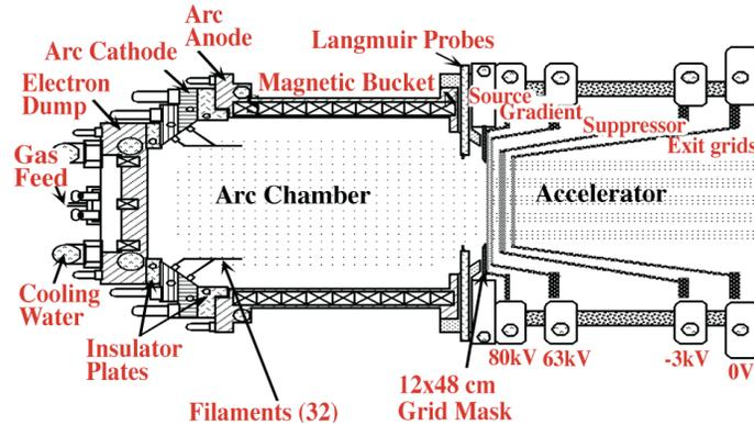
Fig. 2. Cutaway view of a DIII-D ion source.
