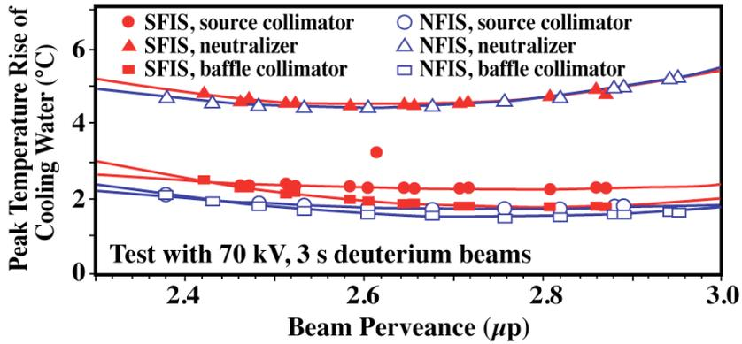
Fig. 12. Peak temperature rise of cooling water for source collimator, neutralizer, and baffle collimator.
