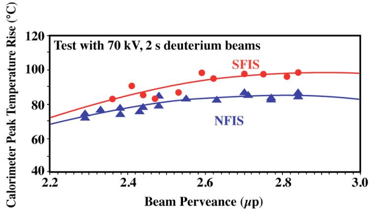
Fig. 11. Calorimeter temperature rise.
