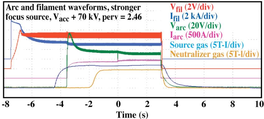
Fig. 7. Waveforms of an arc discharge.
