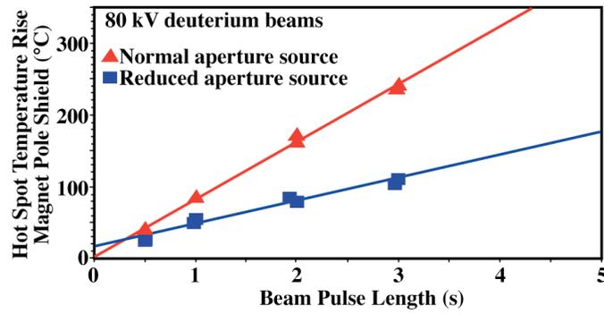
Fig. 4. Magnet pole shield peak temperature rise as function of beam pulse length.
