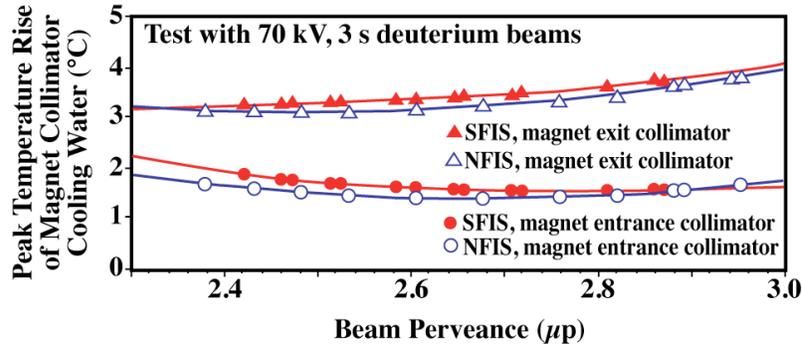
Fig. 13. Peak temperature rise of cooling water for magnet collimators.
