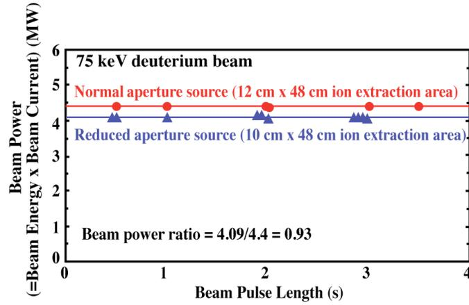
Fig. 3. Beam power comparison for the reduced aperture and normal aperture sources.
