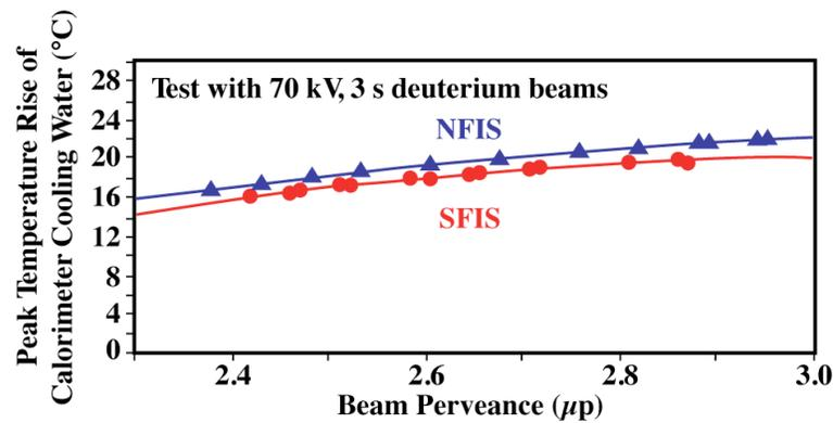
Fig. 14. Peak temperature rise of cooling water for calorimeter.
