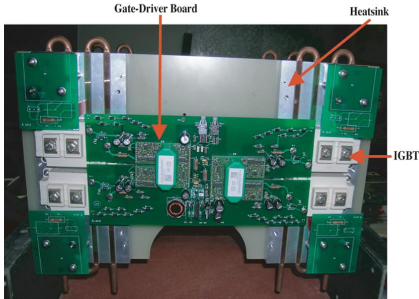
Fig. 2. Assembled IGBT modules successfully demonstrated proper high voltage switching.
