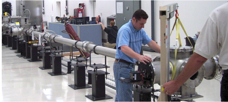
Fig. 5. Full-scale IFE power plant target injection/tracking experiment.
