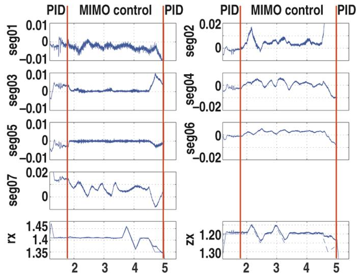
Fig. 3. Experimental shape control results in shot 123357. Segment 1 through 7 plots represent error signals at target isoflux control points.
