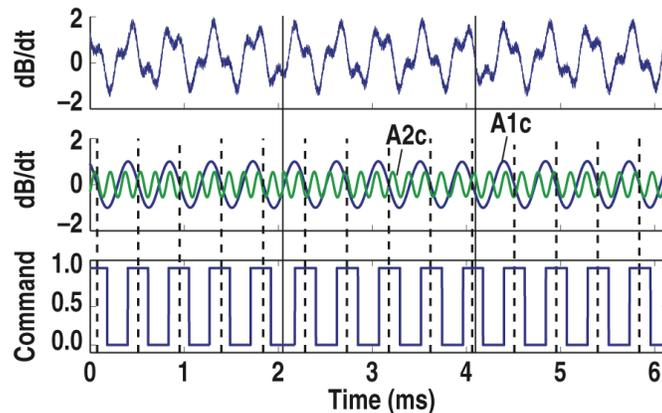
Fig. 1. Simulation of synchronization of gyrotron commands with 2/1 NTM: (a) derivative of magnetic probe signal, (b) extracted 2/1 and 3/2 NTM signals, (c) commands to gyrotrons to suppress 2/1 mode.
