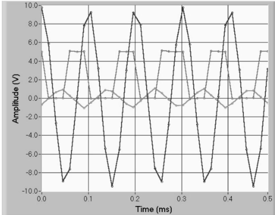
Fig. 3. 10 kHz sine, square, and triangular signals are sufficiently well represented when sampled at 66.8 kHz.
