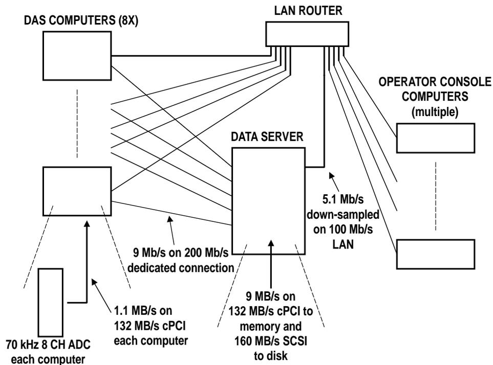
Fig. 1. Network topology and data stream rates.
