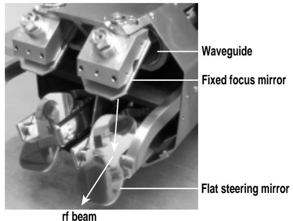
Fig. 3. A high speed dual launcher with two axis movement for each rf beam.
