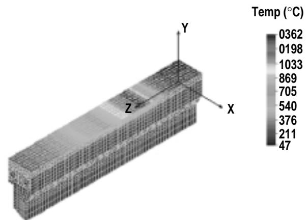
Fig. 4. Temperature distribution on surface of the divertor.
