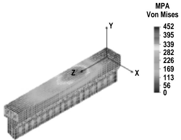
Fig. 5. Stress distribution in the heat sink.
