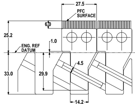
Fig. 2. Attachment concept to join copper fingers to support structure.
