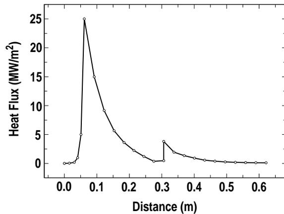
*Fig. 3. Axial distribution of heat flux on divertor surface.*
