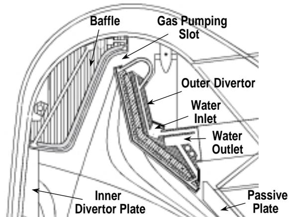
Fig. 1. Cross section through FIRE divertor and baffle.
