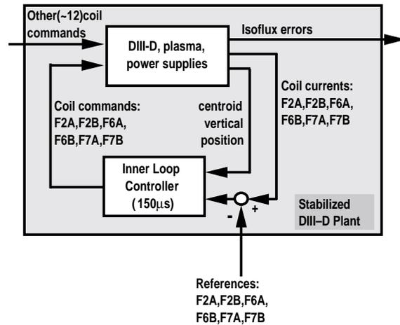
Fig. 3. Simultaneous stabilization and control of current in vertical control coils.
