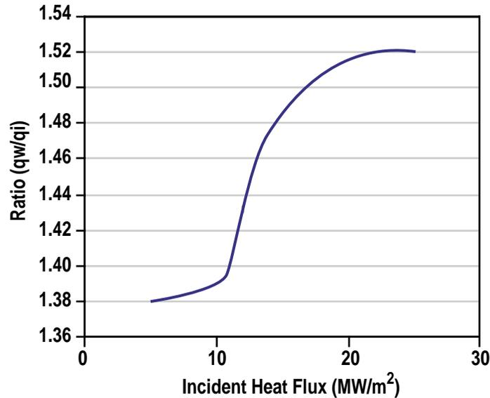
Fig. 3. Ratio of incident heat flux to wall heat flux as a function of incident heat flux.
