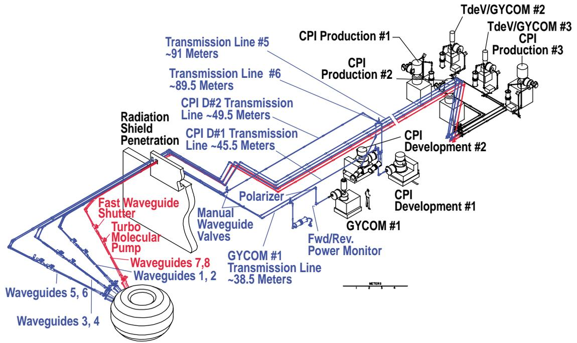
Fig. 1. ECH transmission line layout and configuration.
