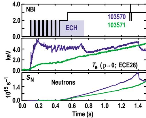
Fig. 3. Enhancements in  $T_e$  and  $S_n$  after ECH turnoff.
