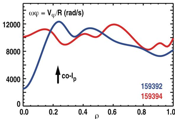
FIGURE 5. Toroidal rotation profiles for the higher power time, with a reduction in the near-axis rotation for the more on-axis deposition ECH discharge.
