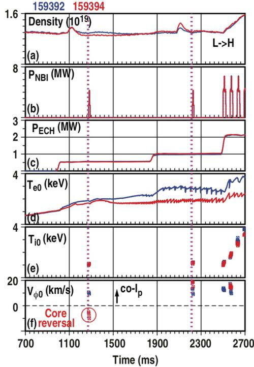
**FIGURE 1.** Time traces of two discharges with differing ECH deposition locations. (a) line averaged electron density (b) NBI blip power (c) ECH power steps (d) Core electron temperature (e) core ion temperature (f) core toroidal velocity.
