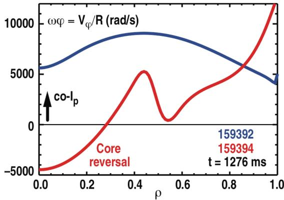
FIGURE 3. Toroidal rotation profiles for the low power time, with reversal in the off-axis deposition ECH discharge.
