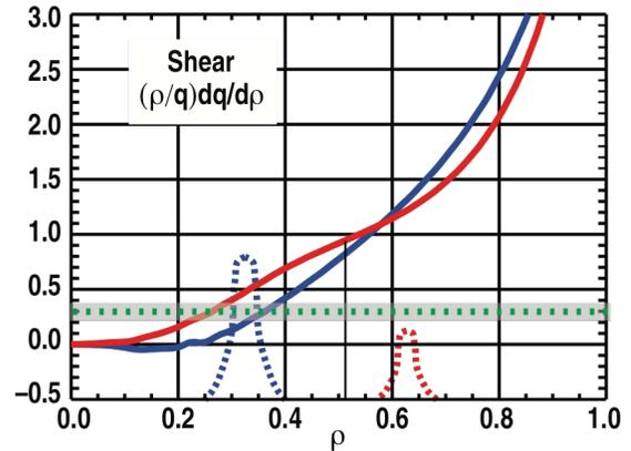
FIGURE 4. Normalized q-profile shear with the deposition locations indicated (au). The horizontal dashed line is at a critical value in the shear from ref [9].
