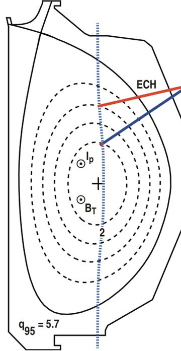
**FIGURE 2.** ECH power ray traces; absorption on the near vertical 2<sup>nd</sup> harmonic surface. The surfaces are constant  $\rho$ . The color code is the same as in Fig. 1.
