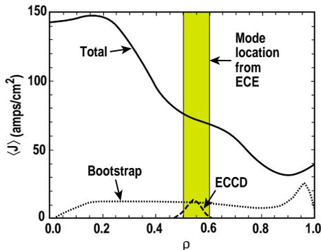
**Figure 3.** Profiles of the total flux-surface averaged (solid), bootstrap (dotted), and ECCD (dashed) current densities versus normalized radius. The shaded region shows the location of the mode as determined from ECE.
