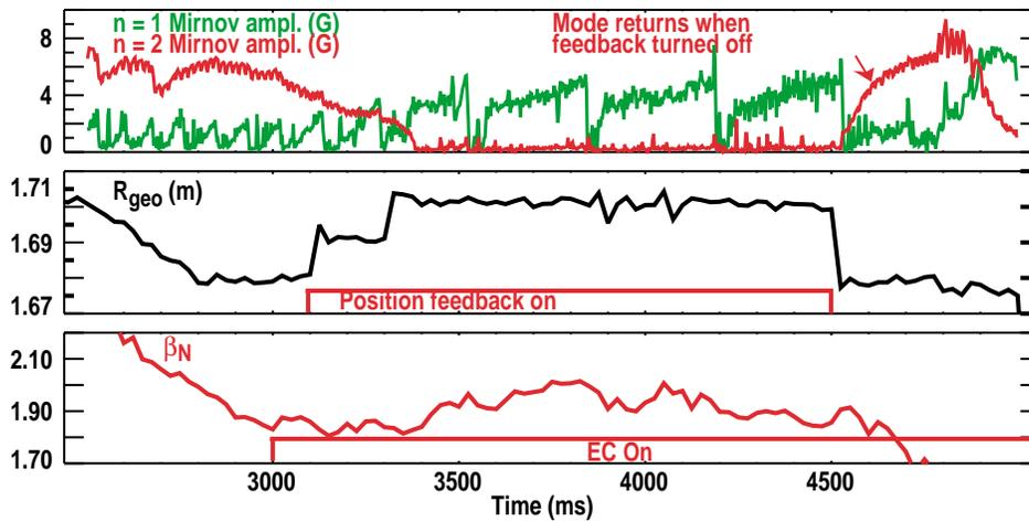
**Figure 6.** Time histories of (a)  $n=2$  (dark) and  $n=1$  (light) Mirnov amplitudes (G), (b) major radius (m), and (c)  $\beta_N$ . The plasma conditions are  $B_T = 1.53$  T,  $I_p = 1.08$  MA,  $\bar{n} = 3.5 \times 10^{19} \text{ m}^{-3}$ ,  $q_{95} = 3.6$ , and  $P_{EC} = 1.5$  MW.
