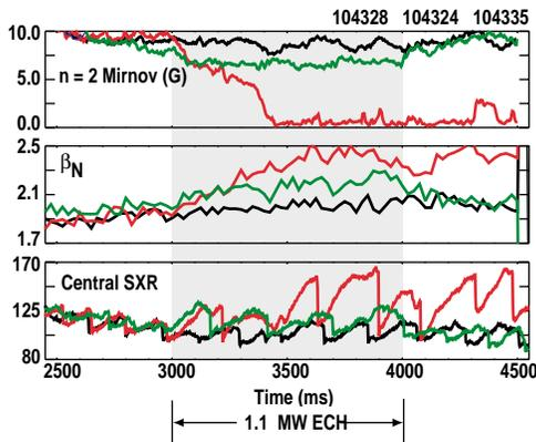
**Figure 1.** Time histories of the (a)  $n=2$  Mirnov amplitude (G), (b)  $\beta_N$ , and (c) central SXR emission (au) for discharges with ECCD at the optimal location (solid), ECCD 2 cm off optimal (dashed), and without ECCD. The EC is applied from 3000–4000 ms (shaded) at 1.1 MW. The plasma conditions are  $B_T = 1.49$  T,  $I_p = 1.18$  MA,  $\bar{n} = 4.1 \times 10^{19} \text{ m}^{-3}$ ,  $P_{NB} = 5.9$  MW.
