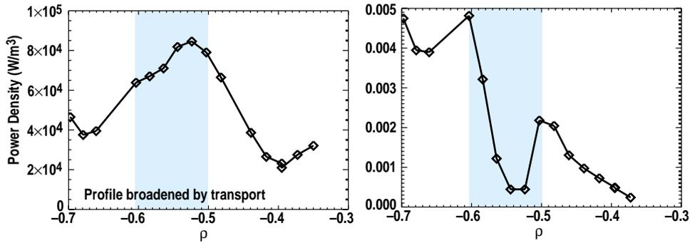
**Figure 5.** Comparison of the locations of the deposited EC power density (100 Hz modulation) and the fluctuating  $\delta T$  (12.5 kHz) due to the tearing mode versus normalized radius.
