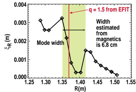
**Figure 4.** Mode displacement  $\xi$  from ECE versus major radius. The value of  $\xi$  is determined from  $\xi \cdot \nabla T = \delta T$ , where  $\delta T$  is measured by the ECE and  $\nabla T$  is the unperturbed profile.
