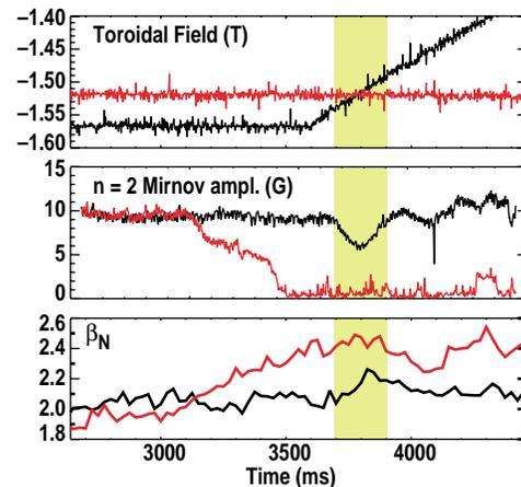
**Figure 2.** Time histories of (a)  $B_T$  (T), (b)  $n=2$  Mirnov amplitude (G), and (c)  $\beta_N$  for a case with a  $B_T$  ramp (dark) and steady  $B_T$  at the maximum effect point (light). The shaded region shows the  $B_T$  values for which the ECCD has an influence. Other than  $B_T$  the conditions are the same as for Fig. 1.
