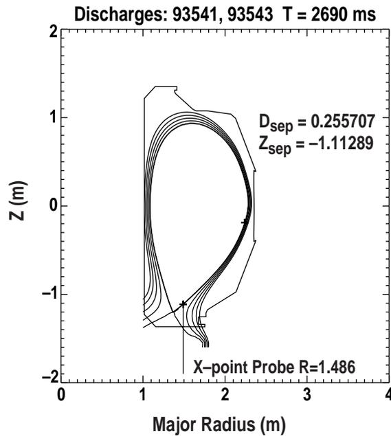
Fig. 1. The position of the scanning probe is superimposed on the reconstructed magnetic geometry for H-mode discharges. The probe moves along the outer SOL.
