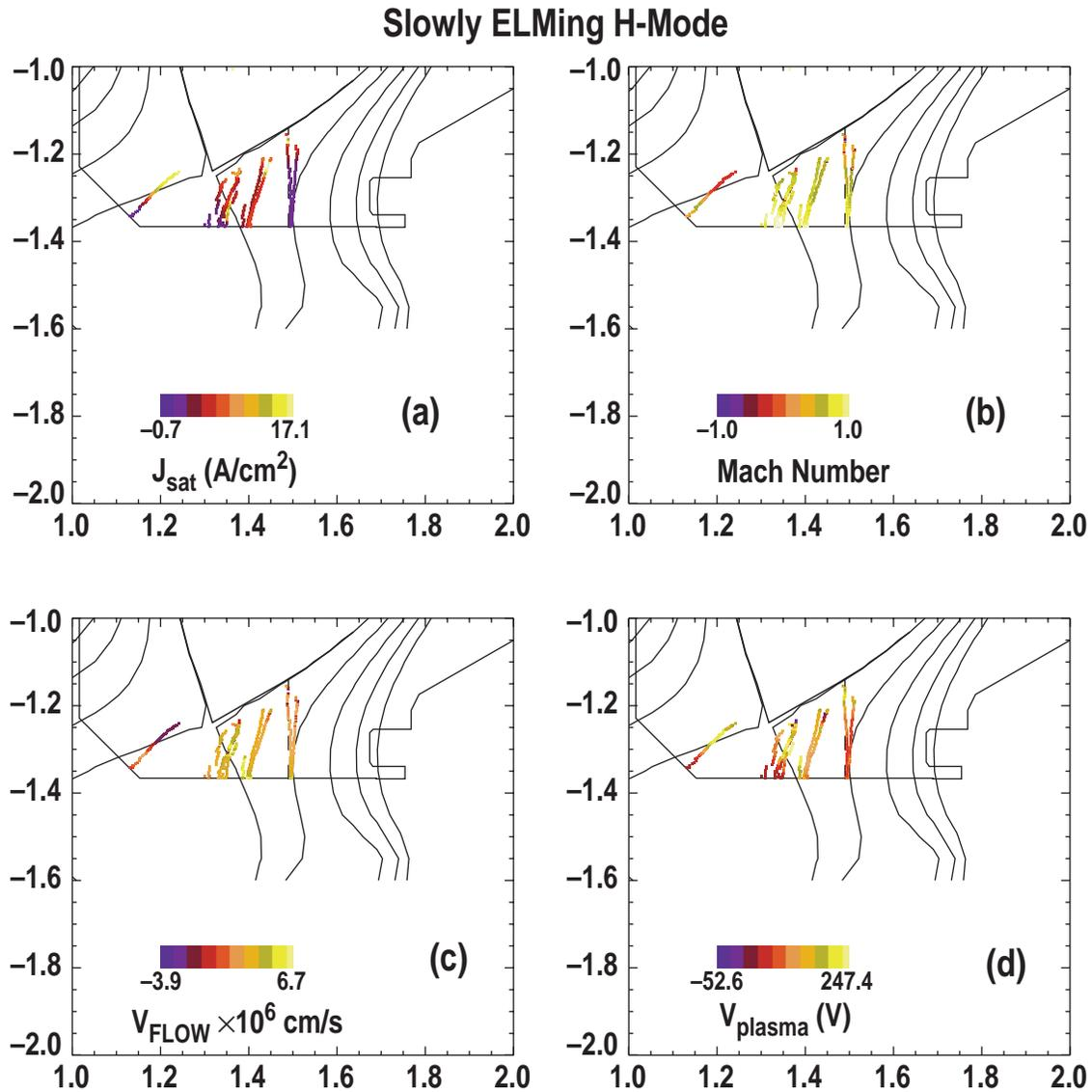
Fig. 3. 2-D plot built over the slowly ELMing phase of several discharges of (a) Ion saturation current, (b) Mach number, (c) Flow velocity and (d) Plasma potential.
