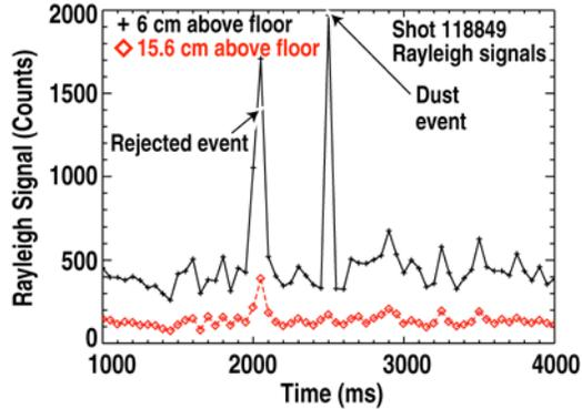
Fig. 2. The Rayleigh channel signal as a function of time is shown for two spatial channels for the plasma shown in Fig. 1. The event at 2500 ms is recorded as a dust event, but the event just after 2000 ms is rejected because it was observed in several spatial channels simultaneously.
