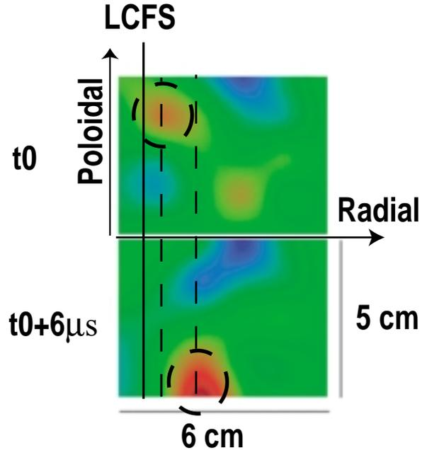
Fig. 4. Two frames from BES showing 2-D density plots. There is a time difference of  $6 \mu s$  between frames. A particular structure is marked with a dashed circle, and shown in both frames, clearly highlighting poloidal and radial motion.
