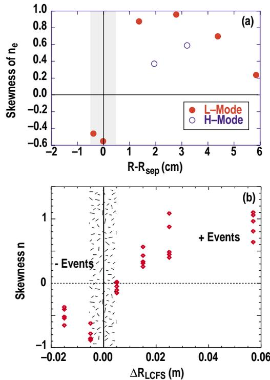
Fig. 5. The skewness of: (a) the  $I_{sat}$  signal, and (b) the BES signal is shown for L-mode (open circles) and H-mode (solid circles) discharge conditions, showing marked deviation from Gaussian behavior. The skewness reverses roughly at the LCFS.
