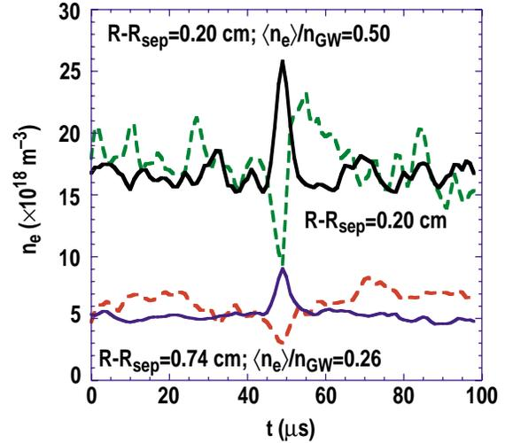
Fig. 6. Conditional averaging of the probe density signals near the LCFS for  $\langle n_e \rangle / n_{GW} = 0.27$  and  $0.5$  indicate the existence of density holes concomitantly with IPOs in that region. This data supports the paradigm of the IPO creation near the LCFS.
