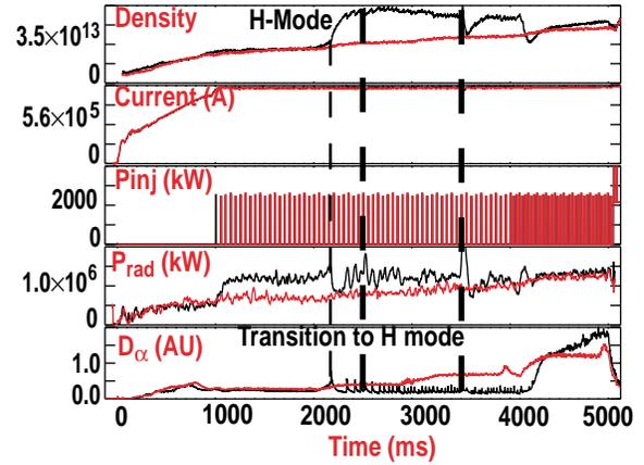
Fig. 1. Time evolution of two discharges in DIII-D showing from top to bottom, density, plasma current, injected power, radiated power and  $D_\alpha$  signals. The transition to H-mode occurs at 2.15 s in one of the discharges. The probe is inserted at the times marked by the two thick vertical lines.
