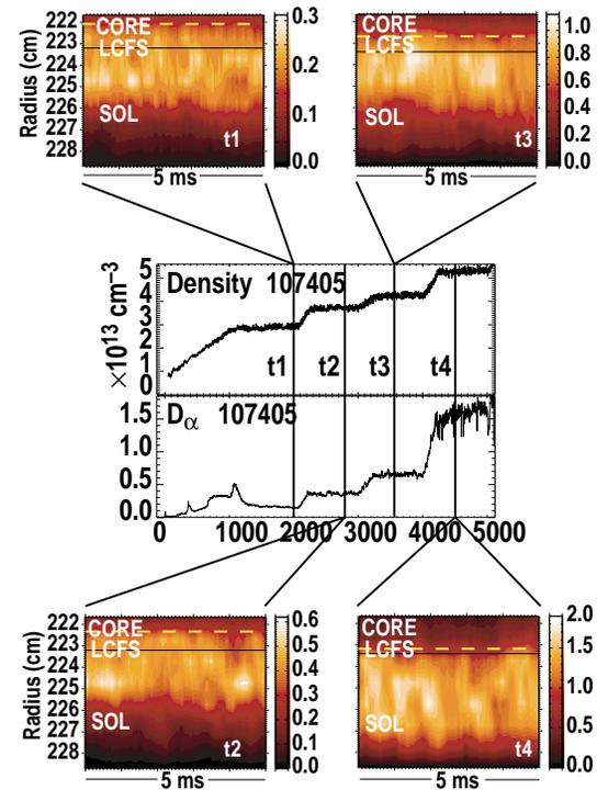
Fig. 3. The time evolution of the L-mode discharge showing the density steps with  $\langle n_e \rangle / n_{GW}$  varying from 0.27 to 0.5. Inserted 2-D plots show the time evolution of the  $D_\alpha$  radial array signals in a 5 ms scale showing the intermittency and its variation with plasma averaged density.
