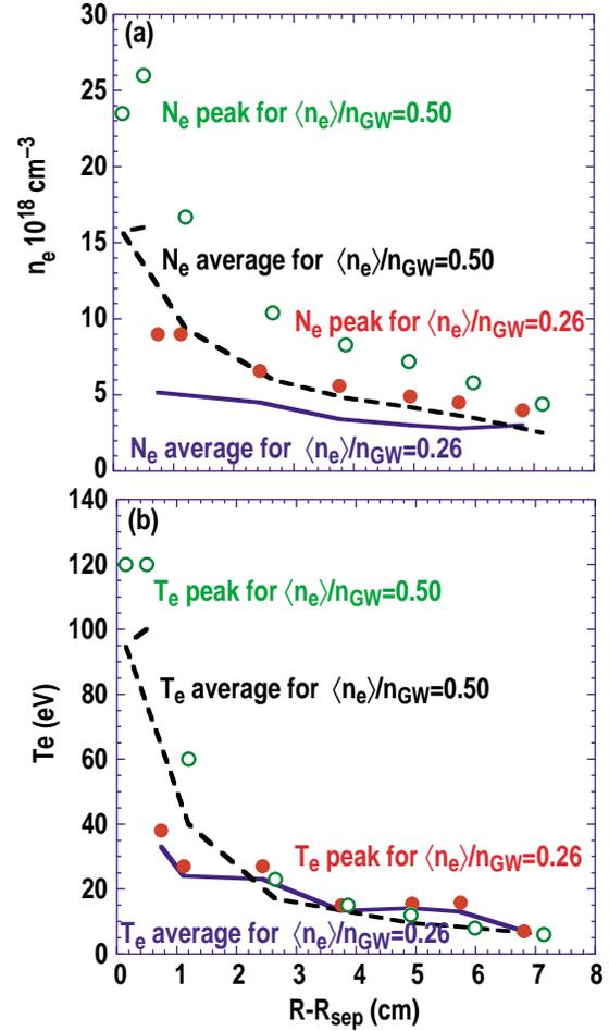
Fig. 8. Radial profiles of (a) the IPO peak density (from conditional averaging) and the average profile and (b) the IPO peak temperature and the average profile for low and high density cases ( $\langle n_e \rangle / n_{GW} = 0.27$  and 0.5). The peak IPO density decays with the same scale length as the background profile while the peak temperature decays much faster.
