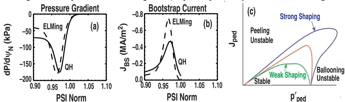
Fig. 1. The edge pressure gradient profiles during the ELMing and QH phases of counter injected discharge 106919 are shown in (a). The edge bootstrap current profile from NCLASS using the measured profiles is shown in (b). A stability diagram for edge localized peeling/ballooning modes derived from the ELITE model is shown in (c).
