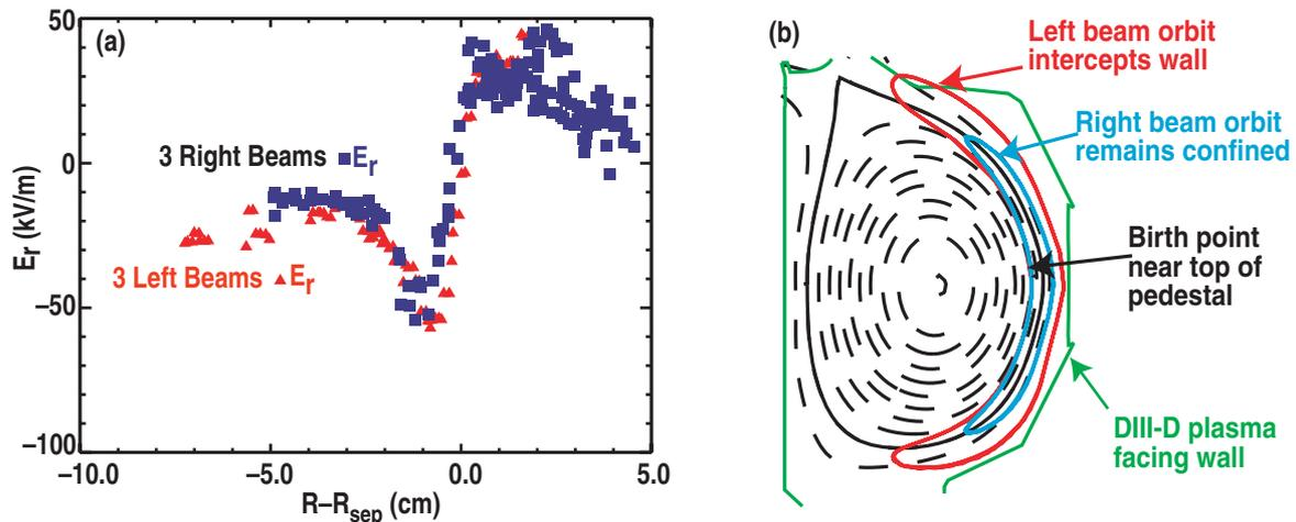
Fig. 2. (a) The edge radial electric field for a QH with (left beams) and without (right beams) prompt fast ion loss. The ELMing phase has a well depth of  $-20$  kV/m. (b) Calculated orbits of beam ions originating near the pedestal during QH mode. Left beams have a tangency radius of 1.2 m, while right beams are tangent at 0.75 m.
