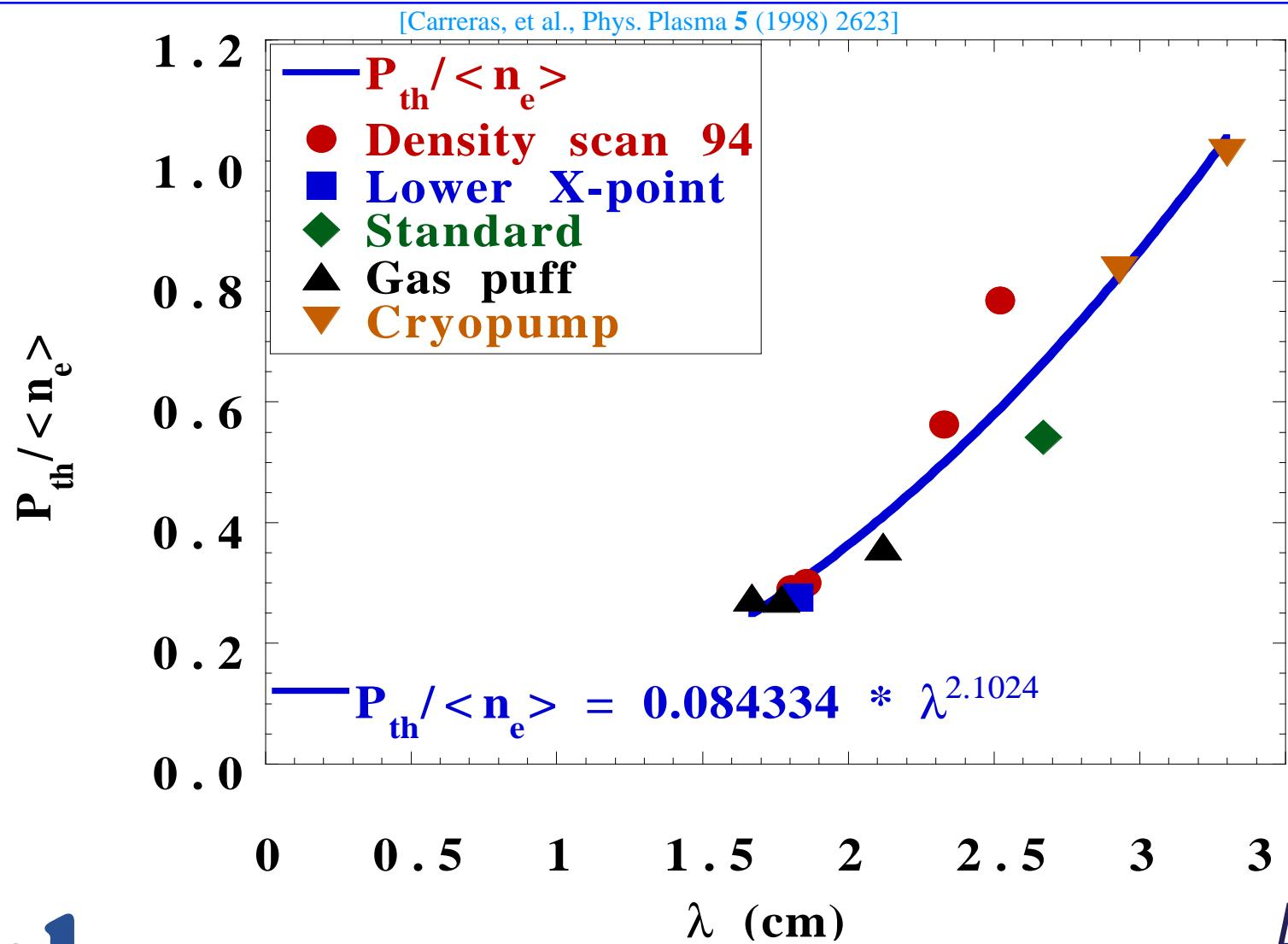
The power threshold correlates with the ratio of the CX damping rate to the neoclassical damping rate (Carreras, PoP 1998)
