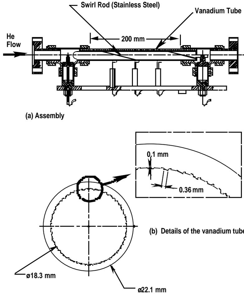
Fig. 1. Details of swirl rod insert (SRI) with 2D roughness for vanadium module.
