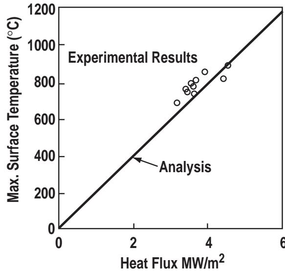
Fig. 2. Comparison of analysis and experiment for SRI with 2D roughness. Vanadium module with a 4 MPa helium coolant pressure.
