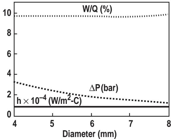
Fig. 3. Performance of a smooth vanadium tube 1 m long and 1.5 mm thick cooled by helium at 4 MPa inlet pressure and 20°C inlet temperature.
