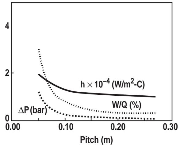
Fig. 4. Effect of pitch on pressure drop, required heat transfer coefficient and pumping power. SRI with 2D roughness with vanadium tube 8 mm diameter. 4 MPa helium pressure and 20°C inlet temperature.
