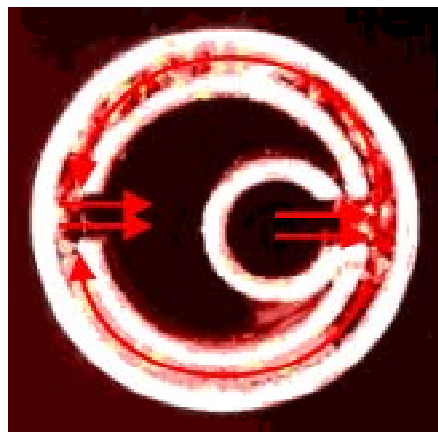
Fig. 2. Thermacore circumferential flow design porous Ta implant.
