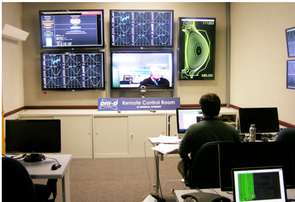
Fig. 2. The remote control room as used during KSTAR operations. Five large TVs face the scientific staff and 6 smaller 24" monitors display plasma control quantities (right).
