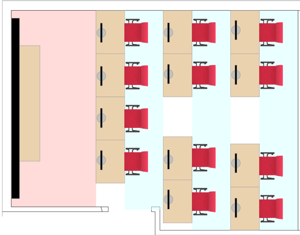
Fig. 1. Remote control room schematic from overhead showing 12 seats available scientific staff. The left side shows 5 TVs and the top shows six 24" LCD monitors.
