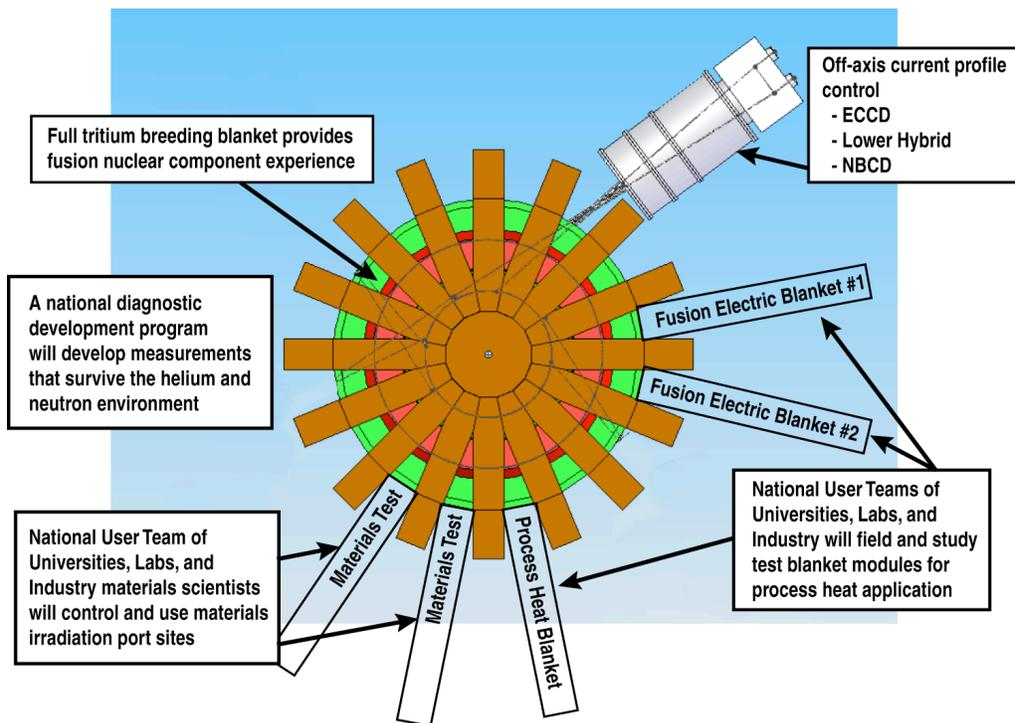
Fig. 3. Current drives and arrangement of different test blankets and test ports.
