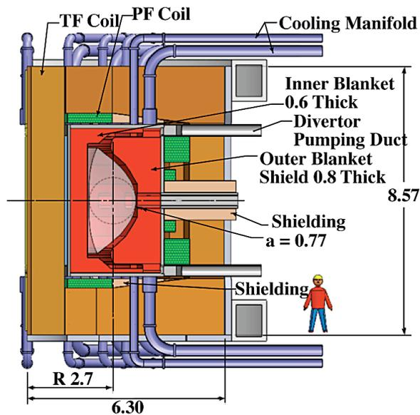
Fig. 1. FNSF-AT schematic showing major radius at 2.7 m, minor radius at 0.77 m, and a machine height of 8.57 m.
