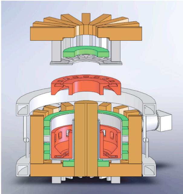
Fig. 2. FNSF-AT baseline maintenance scheme allows crane lift of toroidally continuous ring structures, assuring strength of blankets and precision toroidal alignment of the divertor surface. Red structures are the full blanket assemblies.
