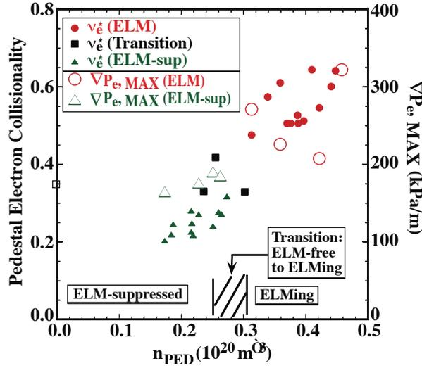
Fig. 3. Electron collisionality and the maximum pressure gradient in the pedestal are plotted versus  $n_{PED}$ .  $\Gamma_{D2} = 0-10 \text{ Pa m}^3/\text{s}$  and  $\Gamma_{Ar} = 0.05 \text{ Pa m}^3/\text{s}$ .
