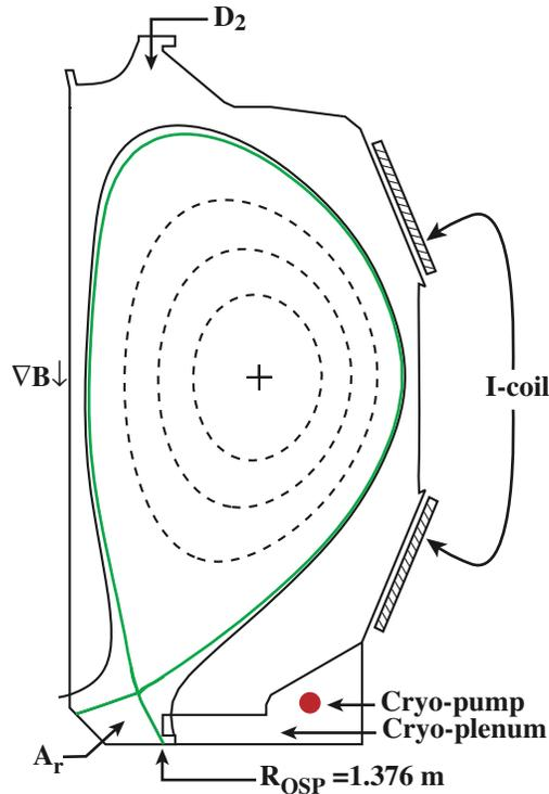
Fig. 1. Unperturbed MHD equilibrium cross-section of the lower single-null configuration with the gas injection, divertor pumping plenum, and RMP I-coil locations superimposed.
