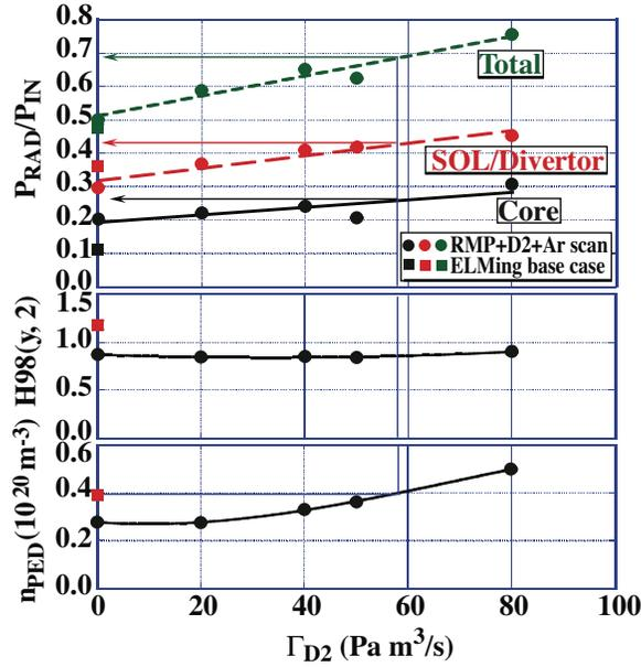
Fig. 5. (a)  $P_{\text{RAD}}/P_{\text{IN}}$ , (b)  $H_{98(y,2)}$ , and (c)  $n_{\text{PED}}$  are plotted versus  $\Gamma_{\text{D2}}$ .  $\Gamma_{\text{Ar}}$  is fixed at  $0.05 \text{ Pa m}^3/\text{s}$ . Data with RMP are shown for a range in  $\Gamma_{\text{D2}}$  (solid circle). The reference case of ELMing without RMP is shown for  $\Gamma_{\text{D2}} = 0$  (solid box). Plasma parameters:  $I_p = 1.43 \text{ MA}$ ,  $q_{95} = 3.5$ , and  $P_{\text{IN}} = 5.4\text{--}6.5 \text{ MW}$ .
