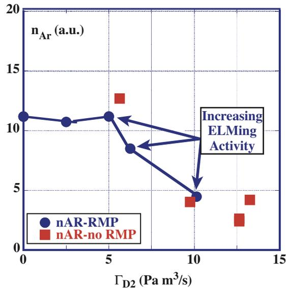
Fig. 4. Relative core argon accumulation in the core plasma ( $n_{Ar}$ ) as a function of  $\Gamma_{D2}$ , in both RMP and non-RMP radiating divertor discharges. The methodology in determining  $n_{Ar}$  is described in Ref. [15].  $\Gamma_{Ar} = 0.05 \text{ Pa m}^3/\text{s}$  in all cases.
