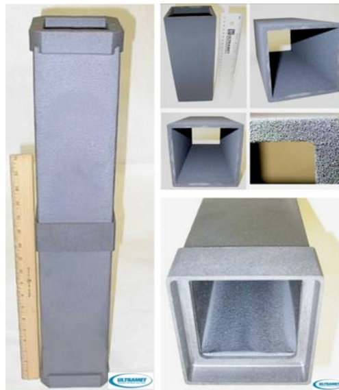
Fig. 4. FCI Prototype consisting of an assembly of two FCI segments totaling a height of 635 mm, 116 mm wide, and 116 mm deep; the SiC-foam was infiltrated by CVD SiC to \sim 10\text{--}20 \text{ vol } \% (Ultramet, Inc.).
