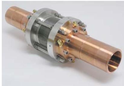
Fig. 4. Prototype of 63.5 mm diameter sliding joint waveguide, shown without protective shield normally surrounding the bellows section.
