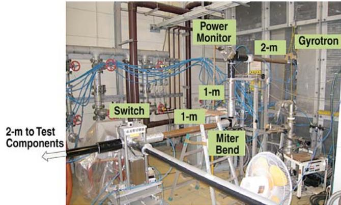
Fig. 1. Layout of the JAEA transmission line before the test section.
