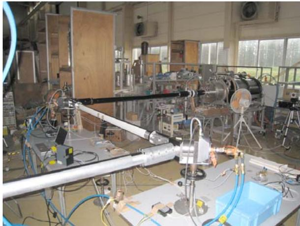
Fig. 2. Configuration for testing the fast rotation polarizer miter bends and dc break.
