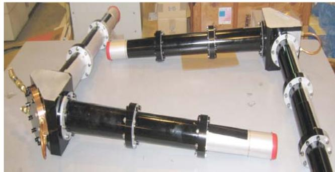
Fig. 3. Pair of low diffraction loss miter bends tested at JAEA test stand. Black tape on surfaces facilitated IR temperature measurements.
