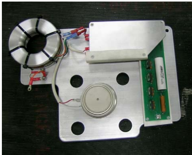
Fig. 2. Photo of single SCR assembly on support plate with triggering and monitoring PCB and toroidal transformer.
