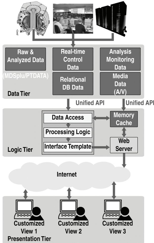
Figure 1. Multi-tier software architecture of DIII-D web-portal.
