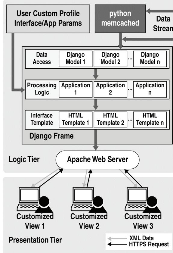
Figure 2. Detailed logic tier and presentation tier.
