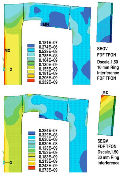
Figure 12. Ring interferences and stresses needed to obtain joint contact.
