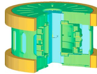
Figure 3. FDF compression joints with ring. The ring is 0.86x2.4 m in this model.
