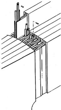
Figure 1. C-Mod sliding TF joint.
