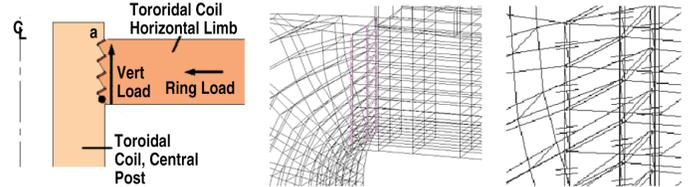
Figure 4. Sawtooth joint and the angled gaps used in the model to represent the sawteeth.
