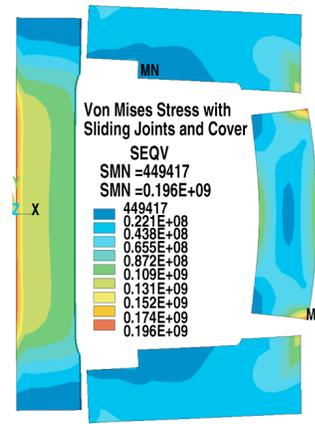
Figure 7. Sliding joints/large cover Von Mises stress max = 0 196 MPa.
