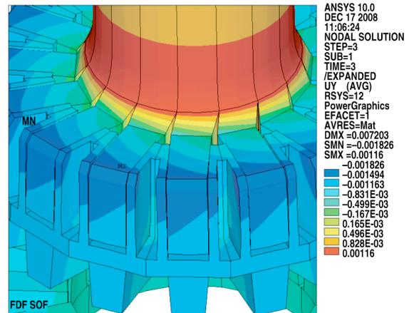
Figure 8. SOF out-of-plane displacements for the sliding joint concept.
