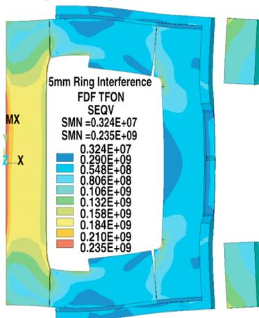
Figure 6. Rebut concept, Von Mises stress – with 0.005 m ring preload, max = 235 MPa.
