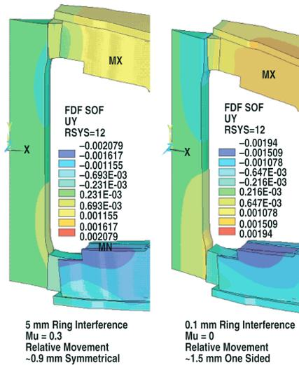
Figure 9. SOF out-of-plane displacements with and without ring preload.
