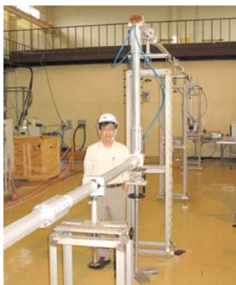
Fig. 3. Transmission line at JAEA 170 GHz gyrotron test stand.
