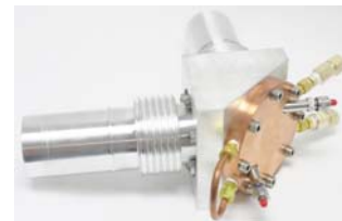
Fig. 2. Miter bend with higher-order mode absorbing sections on miter bend arms.
