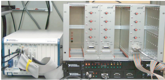
Fig. 1. Filterscope electronics under test. The PXI crate is on the left and the filterscope bin with three modules on the right. The black boxes under the filterscope bin accommodate cabling. The PXI crate contains an Intel CPU, a parallel interface, and two digitizers.
