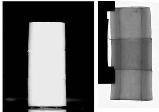
Figure 9. A side view optically and by radiograph of the three section foam annulus. The foam is 15.5 mm tall, 7 mm od, and 4 mm id.
