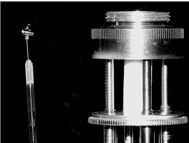
Figure 3. The hohlraum on the left is a full scale Omega target: the hohlraum on the right is a typical dynamic hohlraum without wires. The wires would run through the slots on the top and the bottom of the assembly.
