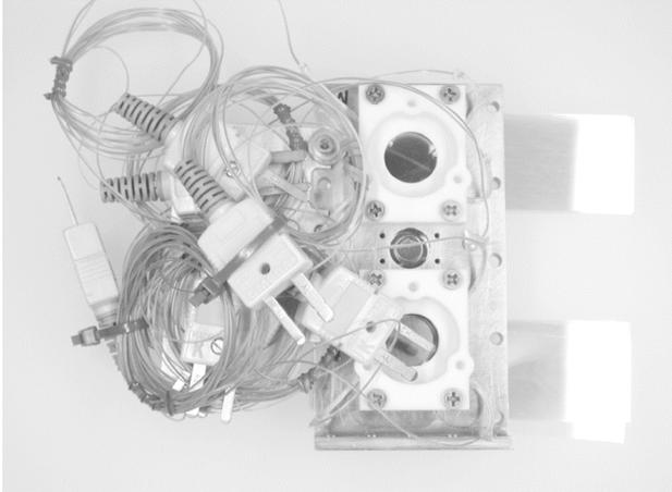
Figure 7. This is one panel of a four panel experiment that was shot on Z. It has two counter bores that have heaters and thermocouples and a center counter bore that has a simple coated window for a velocity measurement.
