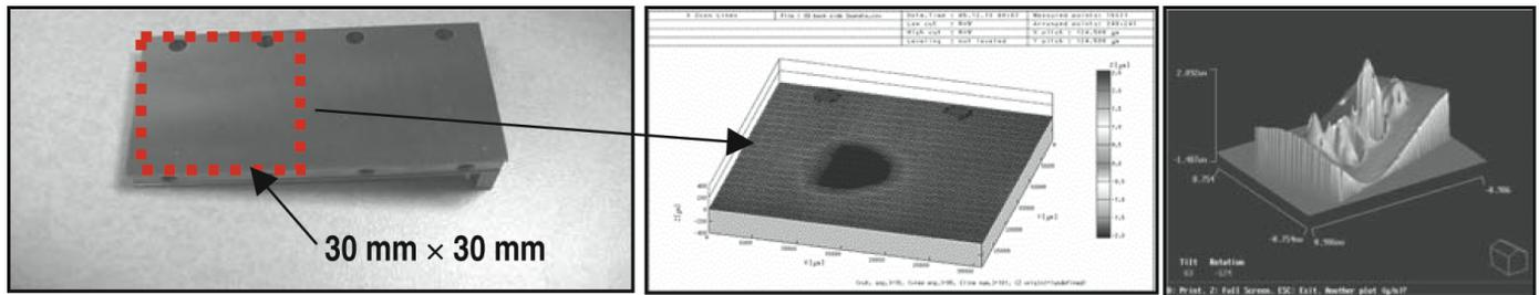
Figure 11. This is a sample analysis of an EOS panel. The power flow surface has a 2.5 micron bow and the counter bore has a ridge 4 microns high.
