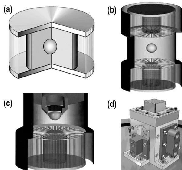
Figure 1. These are four target types typical for Z. The first three are wire array type targets, the fourth is an EOS type. They are: (a) dynamic hohlraum, (b) double pinch hohlraum, (c) fast igniter, and (d) EOS.
