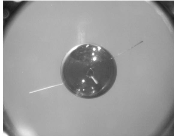
Figure 5. This is capsule with 3 fill tubes mounted in the secondary hohlraum of a double pinch target. The fill tube pointing towards the camera came through a hole in the Formvar film.
