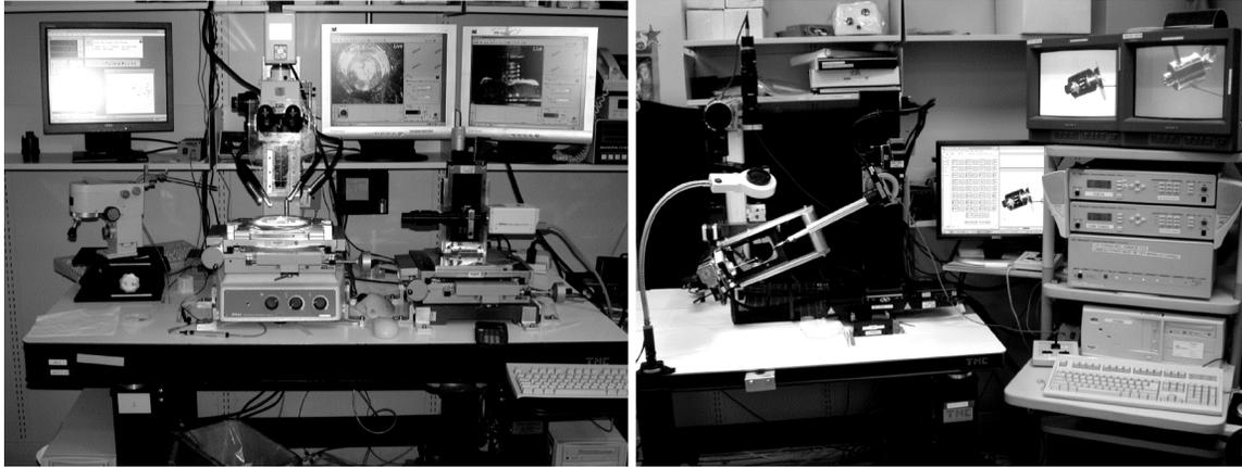
Figure 2. These are the two target fabrication assembly stations. The station on the left has two cameras, a measuring x and y stage and a x measurement on the side camera. The station on the right has the cameras fixed in space to define a cartesian space. The target can move in x, y, z and rotate.
