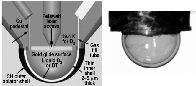
Figure 10. The drawing on the left shows the conceptual components required in the dual hemi cryogenic fast igniter design. The picture on the right shows the prototype target. It has the glide plane components and the two hemispheres.
