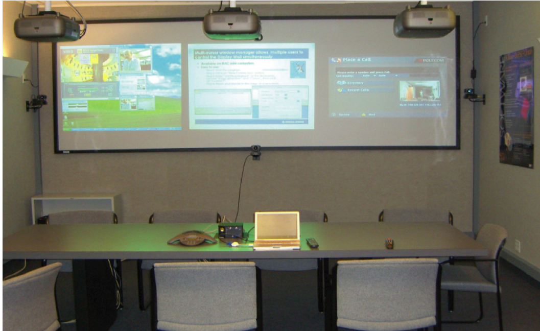
Fig. 3. The three projector screen is shown. On the left, a VRVS-based videoconferencing video is displayed. In the middle a shared presentation is displayed. On the right the Polycom H.323 interface is displayed.
