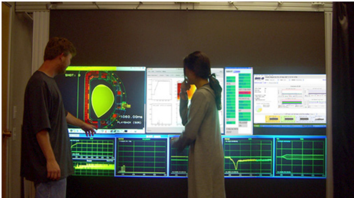
Fig. 2. The 10.5 MPixel high-resolution tiled display demonstrating the remote participation and collaboration tools in the remote control room. The upper half of the tiled display, from left to right, displays the RealTime Boundary Display application, a visualization application window shared from a remote computer via SharedAppVNC, Data Analysis Monitor, and a Ganglia-computational resource monitoring webpage. The lower half of the display shows the streamed video of the PCS signal screens located at DIII-D.
