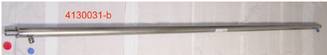
FIG. 2. Stainless steel water jacket around stainless steel waveguide attenuator.
