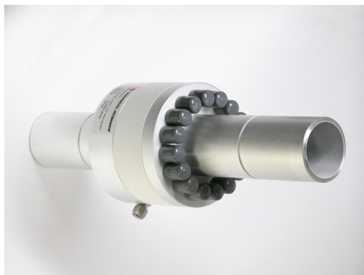
FIG. 5. Prototype ITER 63.5 mm dc break using all ceramic insulators.
