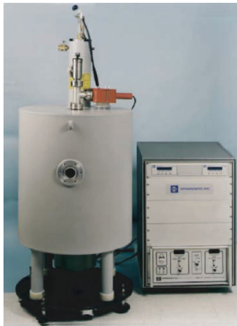
Fig. 19. A DNP NMR Spectrometer using a 460 GHz gyrotron and a 9.4 T superconducting magnet.
