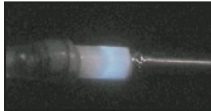
Fig. 7. X-ray catheter developed by LLNL.
