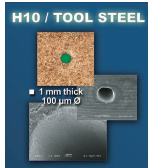
Fig. 13. Laser drilled hole in tool steel using a General Atomics SuperPulse® solid state laser.
