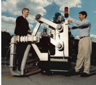
Fig. 16. Concrete surface ablator developed by ORNL using a 56 GHz fusion gyrotron.
