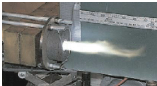
Fig. 15. Microwave powered electrodeless plasma torch developed by MIT.
