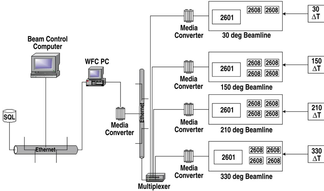
Fig. 1. Block diagram of the water flow calorimetry telemetry system.
