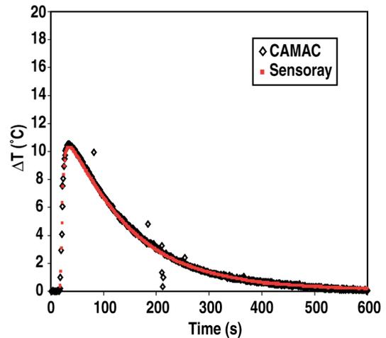
Fig. 6.  $\Delta T$  data for the beam dump calorimeter with ion bending magnet energized.
