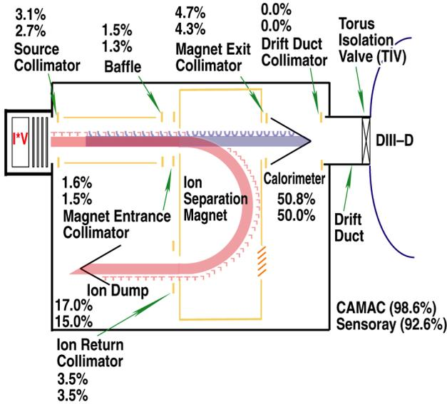
Fig. 8. Power flow accountability comparison with ion bending magnet energized.
