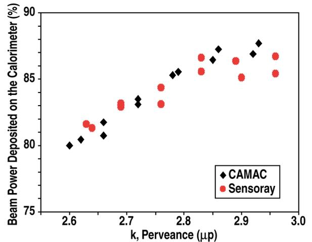
Fig. 2. The measured transmission efficiency.
