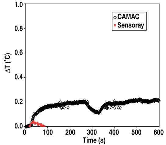
Fig. 5.  $\Delta T$  data for the pole shields with the ion bending magnet not energized.
