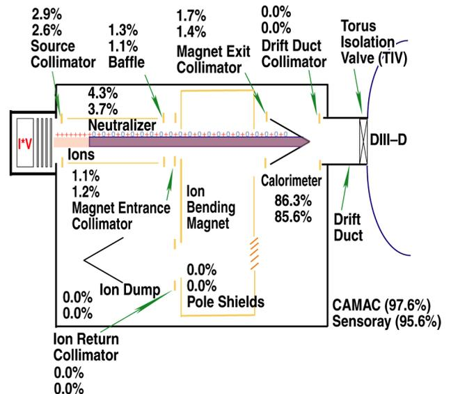
Fig. 3. Power flow accountability comparison ion bending magnet not energized.
