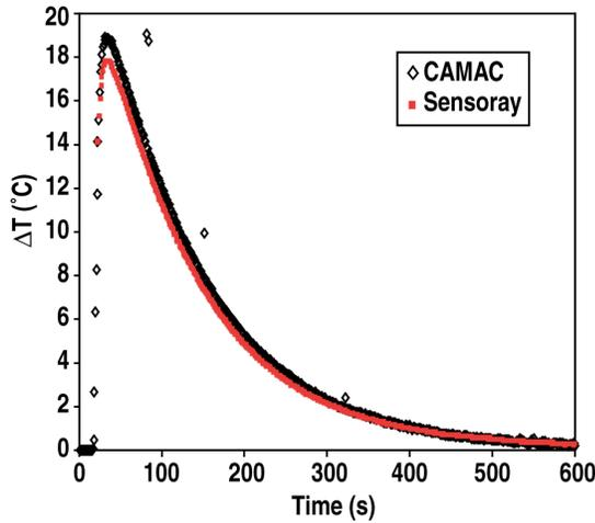
Fig. 4.  $\Delta T$  data for the beam dump calorimeter with ion bending magnet not energized.
