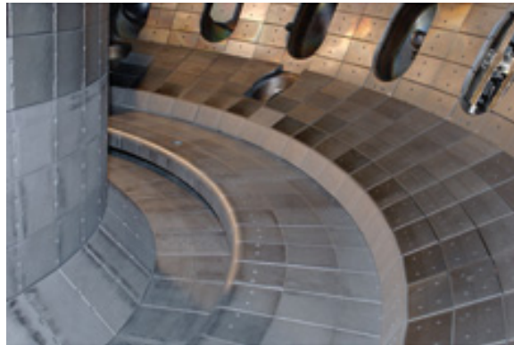
Fig. 1. DIII-D vessel with new lower divertor. A cryopump is located under the outer baffle plate.
