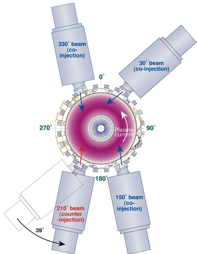
Fig. 1. The 210-deg beamline was rotated to provide the capability for simultaneous co- and counter-injection.
