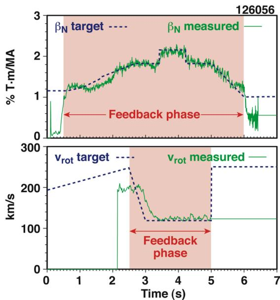
Fig. 6. Simultaneous closed-loop feedback control of stored energy ( $\beta_N$ ) and plasma rotation is demonstrated.
