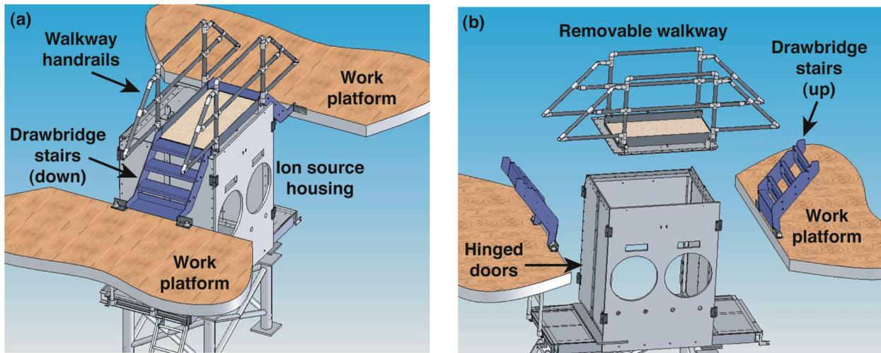
Fig. 4. (a) Modified ion source housing crossover allows access to all areas around perimeter of torus hall. (b) Ion source maintenance or extraction is enabled using removable ceiling (and walkway), drawbridge stairs, and hinged side doors.
