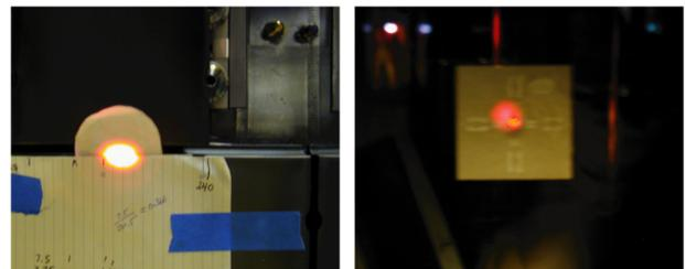
Fig. 5. Laser spots mark beam strike points on targets affixed to vessel wall (left) and to a Plexiglas plate mounted within beam duct near vessel entrance (right).
