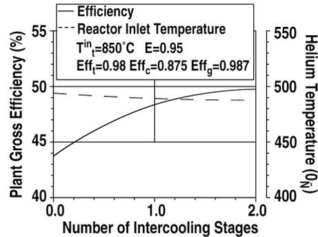
Fig. 10. Impact of intercoolers number on plant efficiency, reactor inlet helium temperature.
