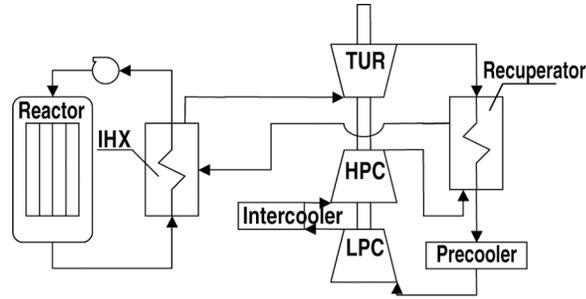
Fig. 6. Indirect cycle GT-MHR flow diagram.
