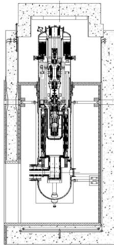
Fig. 7. Layout of the HTR-10GT PCU.
