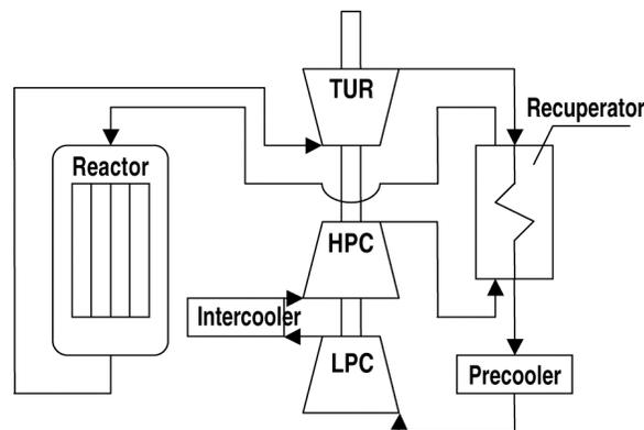
Fig. 5. Direct cycle GT-MHR flow diagram.
