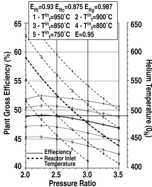
Fig. 1. Impact of reactor outlet helium temperature (at the turbine inlet) on plant efficiency, reactor inlet helium temperature.
