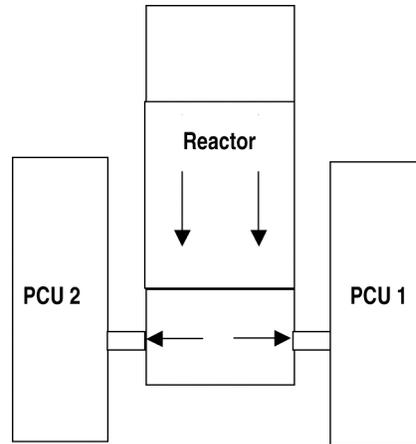
Fig. 11. Flow distribution in lower plenum will be better with 2 PCU design.
