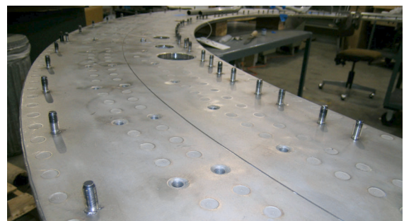
Figure 4. Tile studs on divertor panel.
