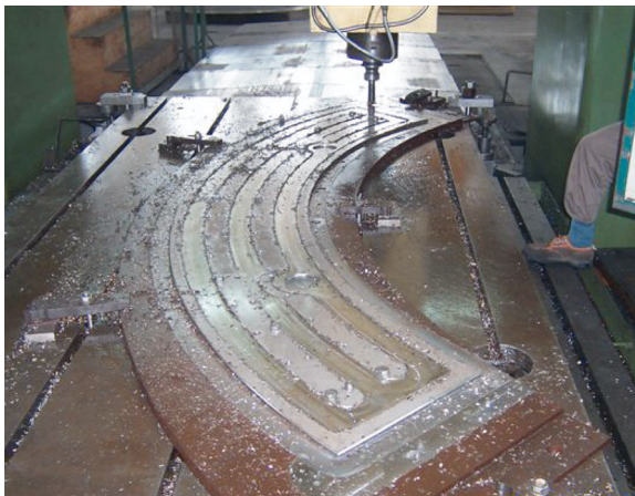
Figure 2. Machining of cooling channels.
