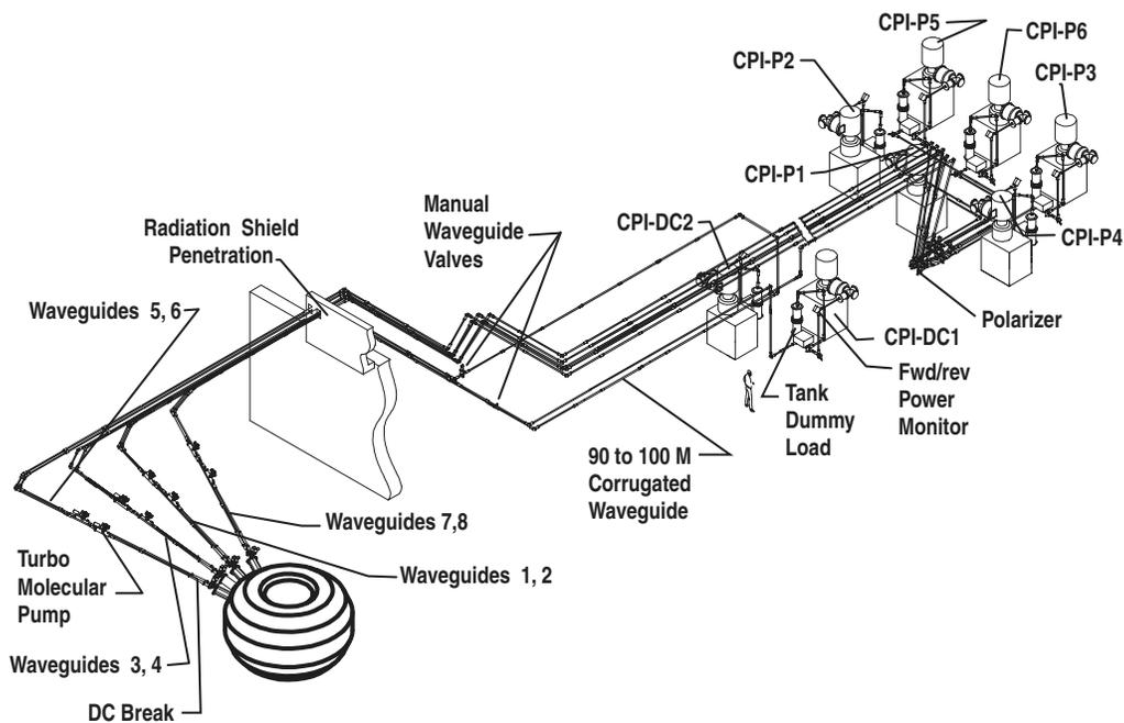
Fig. 2. Layout of the DIII-D EC System as envisioned for 2008.
