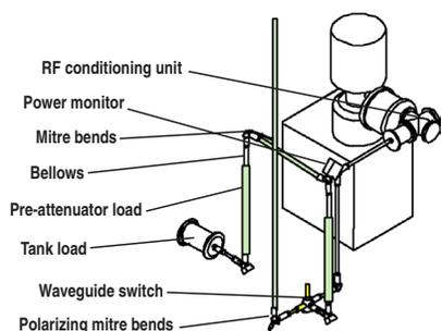
Fig. 3. Configuration of the DIII-D EC system as an ITER EC component test stand, with the major components to be tested identified. All components are 63.5 mm diameter, and evacuated.
