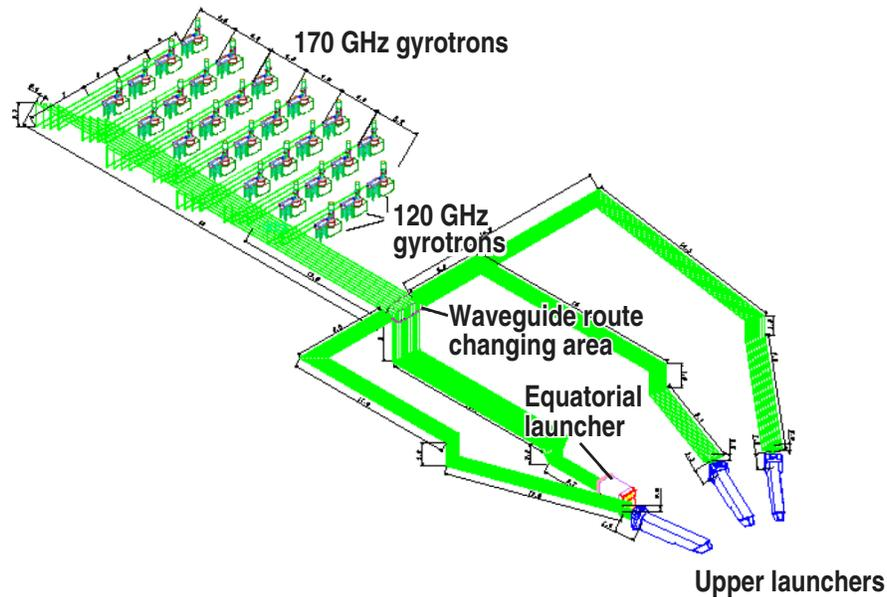
Fig. 1. A layout view of the ITER EC system.
